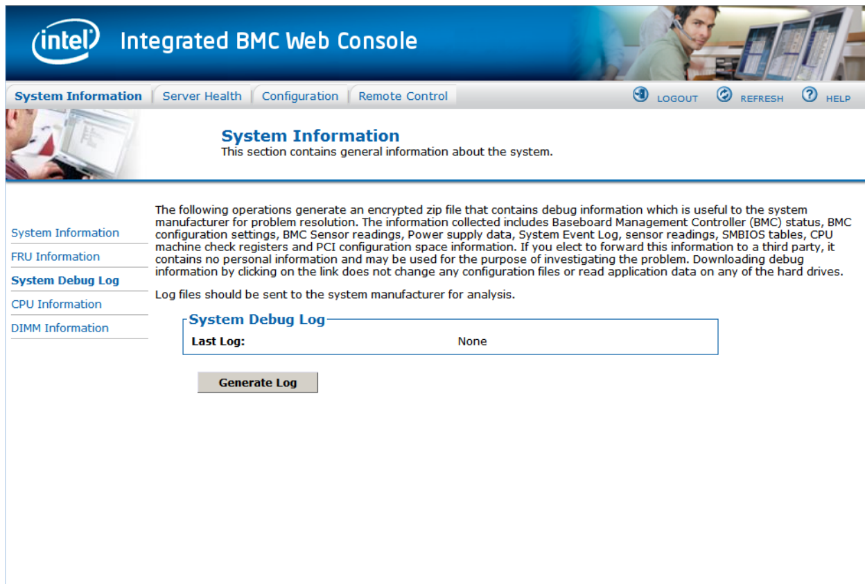
Figure 59: System Information System Debug Log Page on EPSD Platforms Based on Intel® Xeon® Processor E5-4600/2600/2400/1600/1400 Product Families
