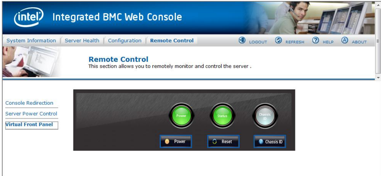
Figure 92: Remote Control Virtual Front Panel Page on EPSD Platforms Based on Intel® Xeon® Processor E5-4600/2600/2400/1600/1400 Product Families
