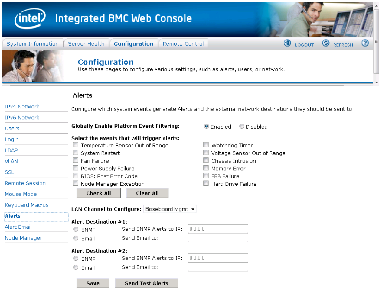
Figure 85: Configuration Alerts Page on EPSSD Platforms Based on Intel® Xeon® Processor E5-4600/2600/2400/1600/1400 Product Families
