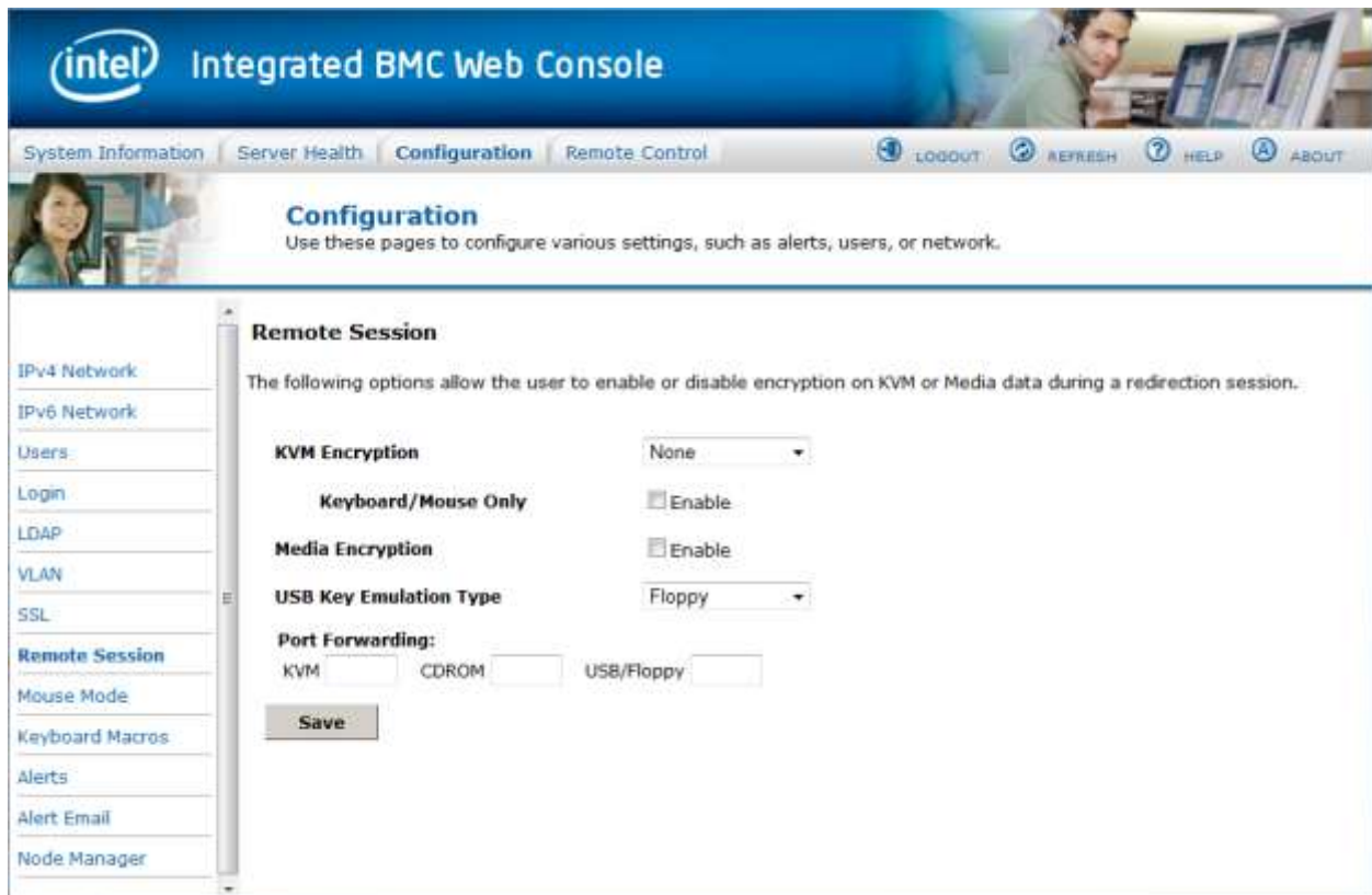
Figure 83: Configuration Remote Session Page on EPSP Platforms Based on Intel® Xeon® Processor E5-4600/2600/2400/1600/1400 Product Families
