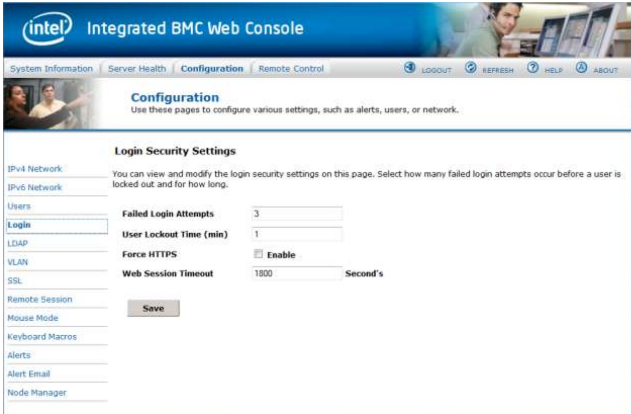
Figure 78: Configuration Login Security Settings Page on EPSD Platforms Based on Intel® Xeon® Processor E5-4600/2600/2400/1600/1400 Product Families and S1200V3RP Product Family
