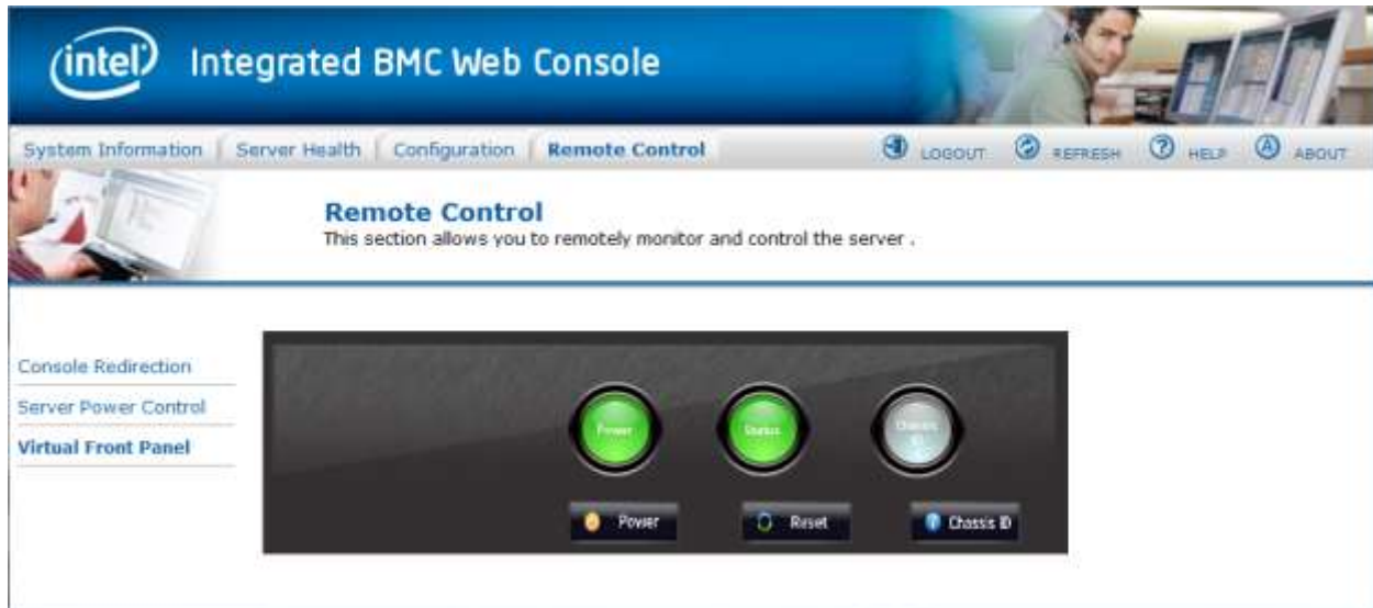
Figure 98: Remote Control Virtual Front Panel Page on EPSP Platforms Based on Intel® Xeon® Processor E5-4600/2600/2400/1600/1400 Product Families and S1200V3RP Product Family
