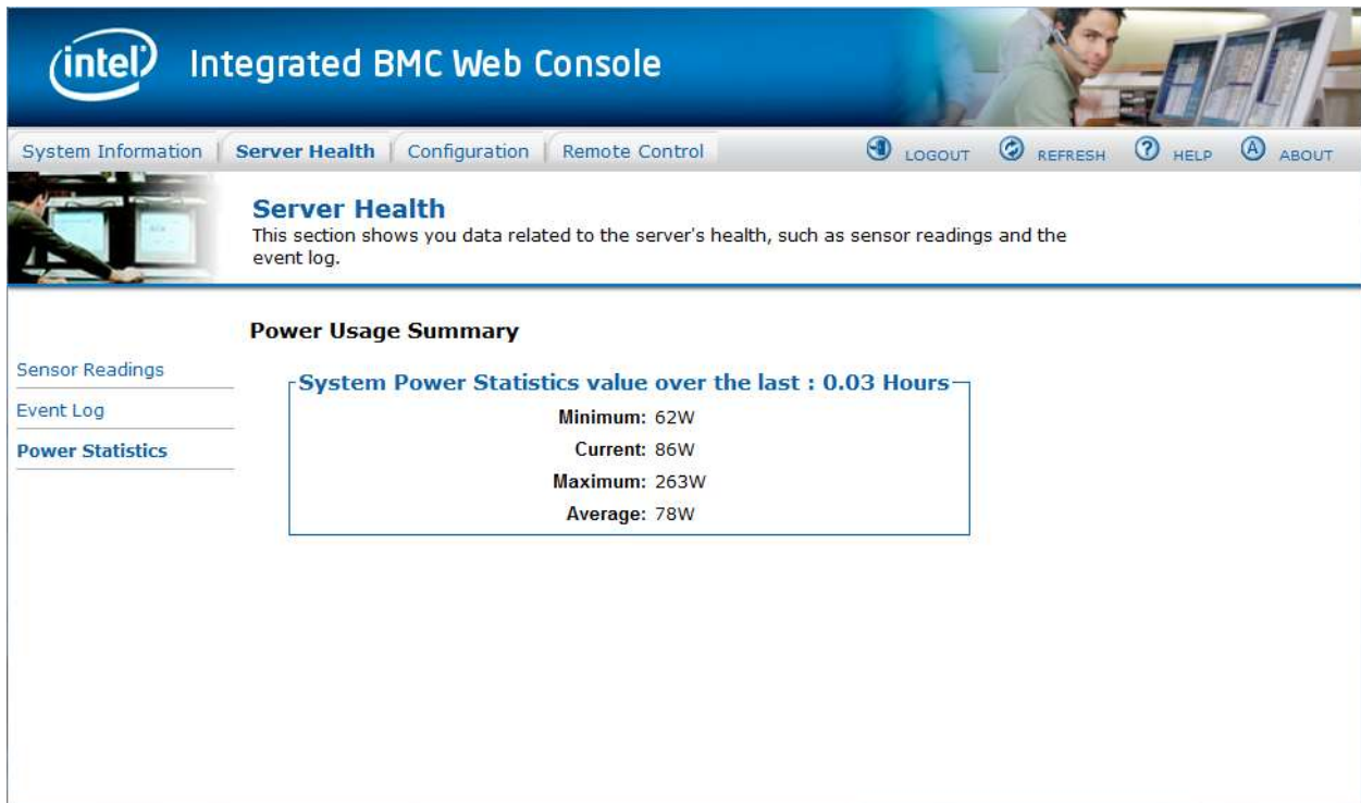
Figure 70: Server Health Power Statistic Page on EPSP Platforms Based on Intel® Xeon® Processor E5-4600/2600/2400/1600/1400 Product Families
