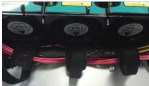
Figure 9. Velcro* Wraps Near Chassis
