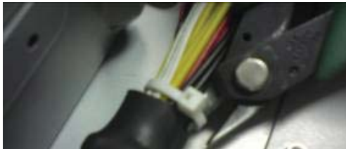
Figure 10. Removing the Cable Tie
