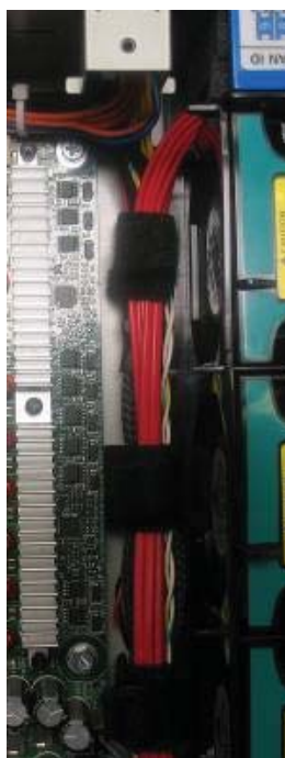
Figure 26. Velcro* Tie Wraps Tucked Into Place
