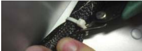
Figure 11. Removing the Cable Tie (Close-Up)
