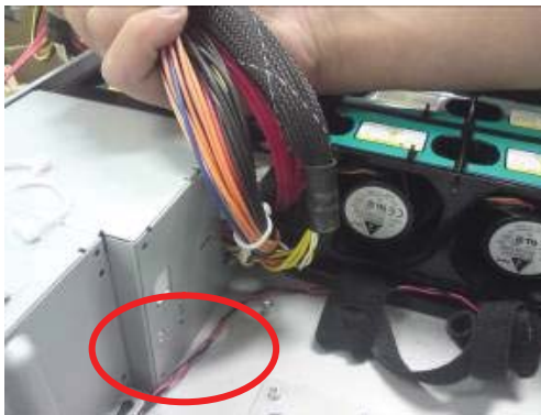
Figure 12. Cable Not Removed From Bundle
