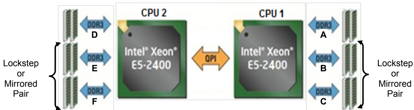
Figure 11. Memory Channel Pairing for RAS Support
