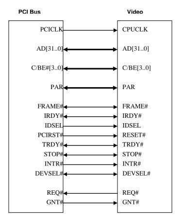
Figure 7. Video Controller PCI Bus Interface
