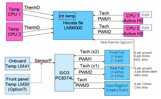
Figure 11. Fan Speed Control Block Diagram
