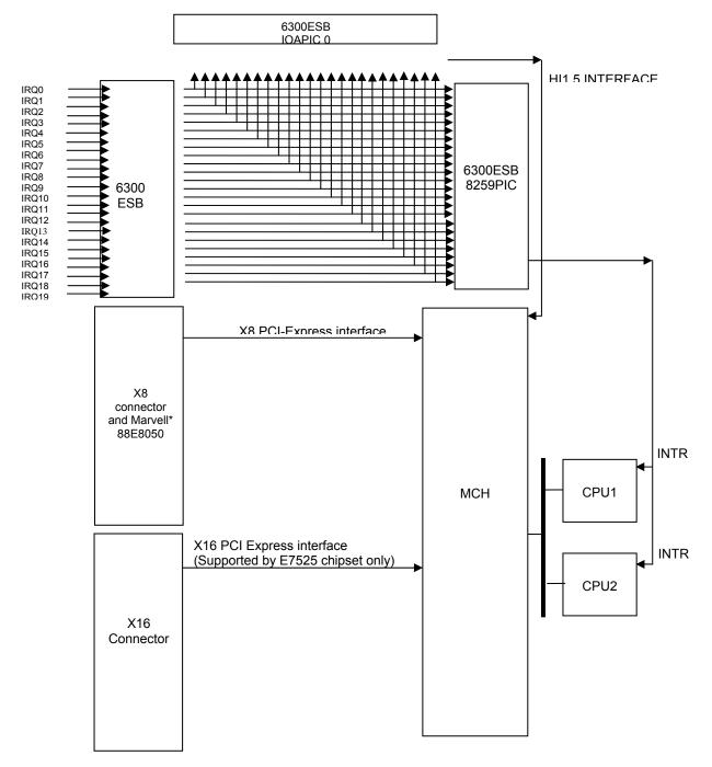
Figure 8. Interrupt Routing Diagram
