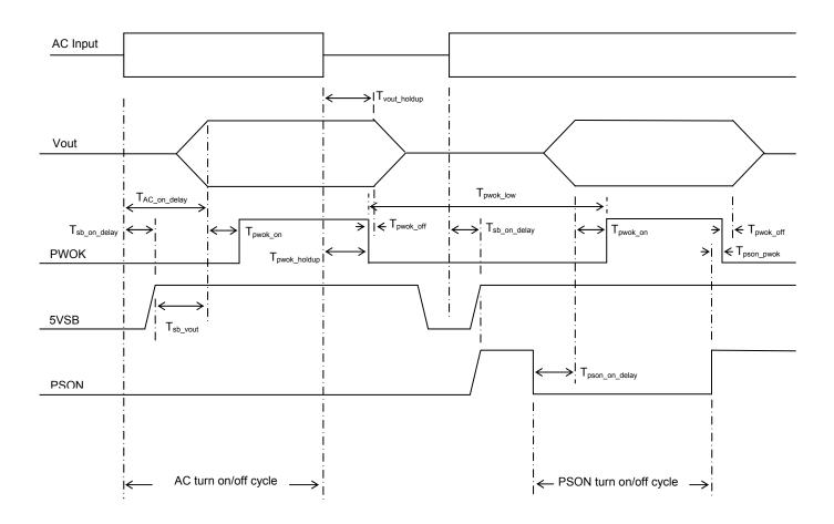
Figure 14. Turn On / Turn Off Timing
