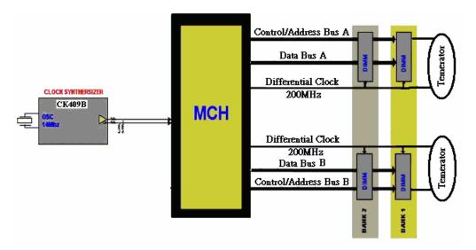
Figure 3. Memory Sub-system Block Diagram
