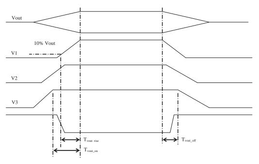
Figure 13. Output Voltage Timing
