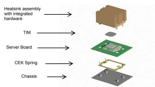
**Note:** When installing either of these server boards into an Intel® Server Chassis SC5300, the passive heatsink solution (no fan) must be used.
