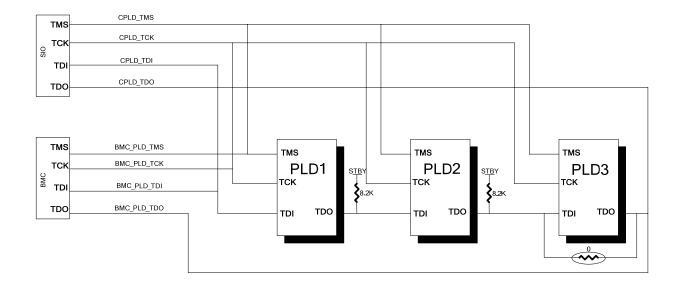
Figure 18. PLD Connections
