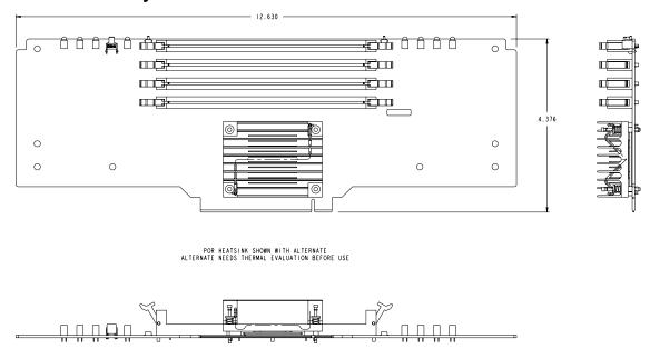
Figure 21. Memory Board Mechanical Outline Drawing
