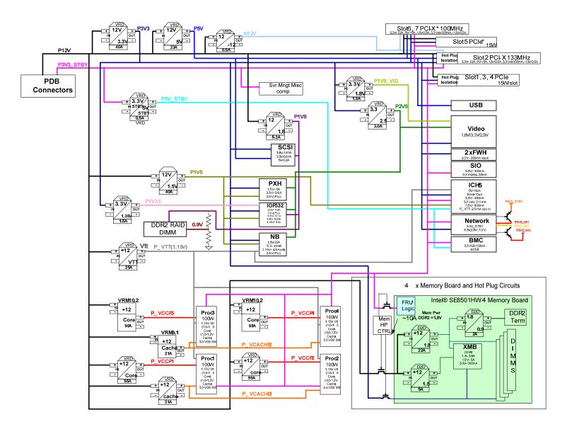
Figure 13. Power Distribution Block Diagram
