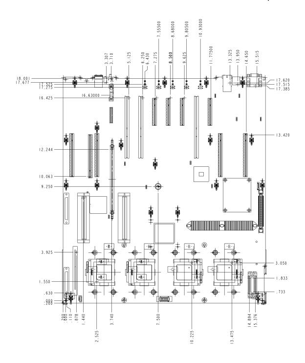
Figure 20. Mainboard Pin 1 Location Drawing
