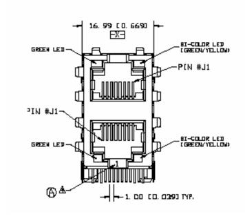
Figure 12. Stacked Ethernet Connector
