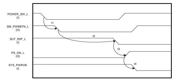
Figure 15. Typical Power-Down Sequence
