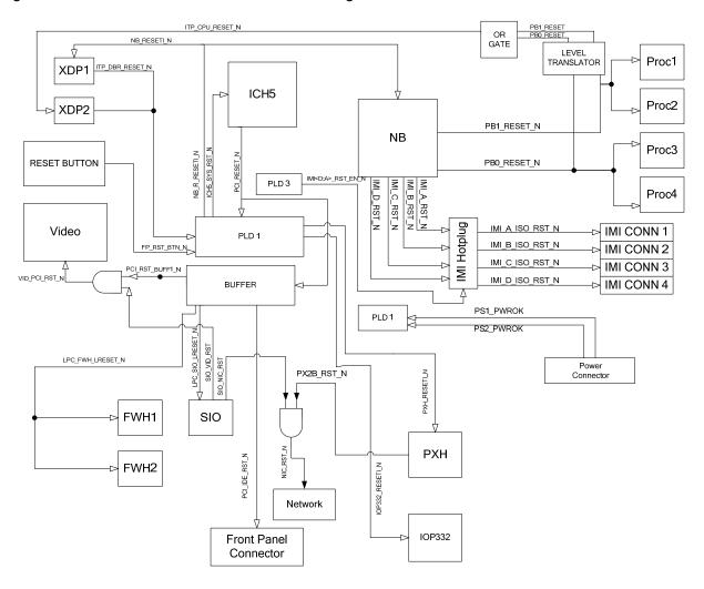
Figure 16. Reset Block Diagram
