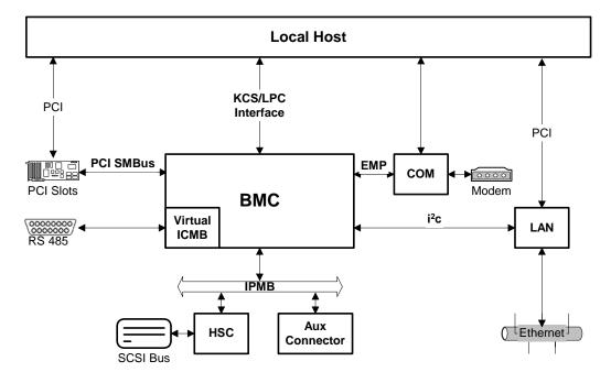
Figure 9. External Interfaces to the BMC
