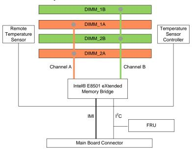
Figure 6. Memory Board Block Diagram
