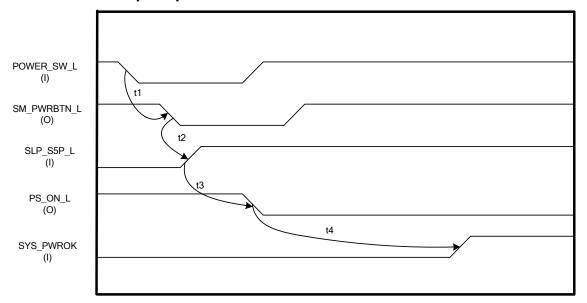
Figure 14. Typical Power-Up Sequence
