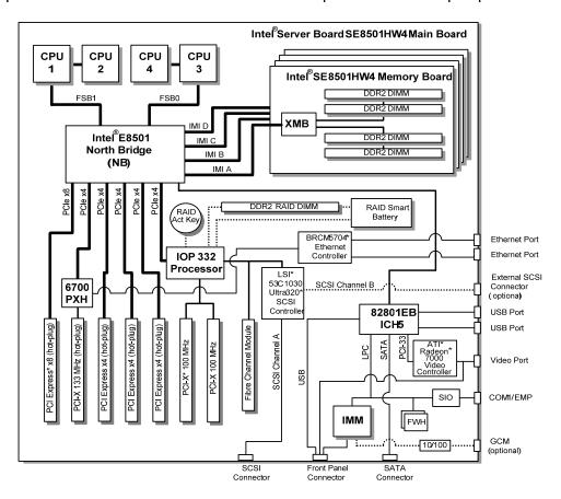
Figure 2. Intel® Server Board Set SE8501HW4 Interconnect Diagram
