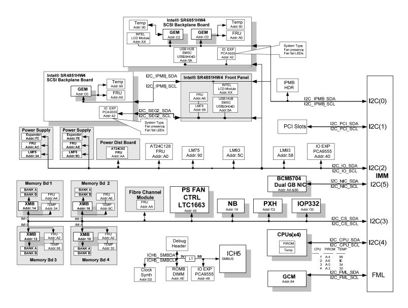
Figure 8. I<sup>2</sup>C Block Diagram
