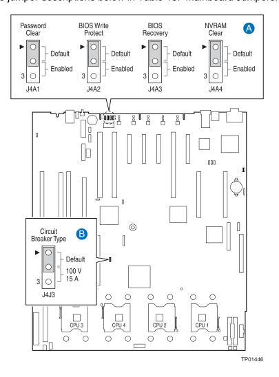
Figure 10. Mainboard Jumper Locations
