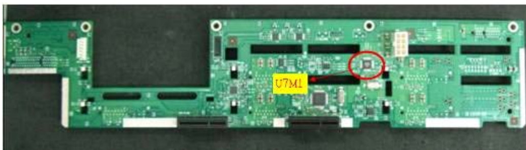
Figure 2: SR2600 Backplane (PBA# E32704-203) - Location U7M1
