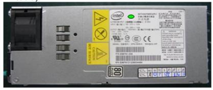
**Phase 2** - The power supply incorporates the first change plus changes of two resistors. This creates an estimated combined margin of 20%. The Power supply version will evolve from E98791-006 to E98791-007 to incorporate both changes. New system builds will include the -007 version and will begin to ship on July 27<sup>th</sup>.
