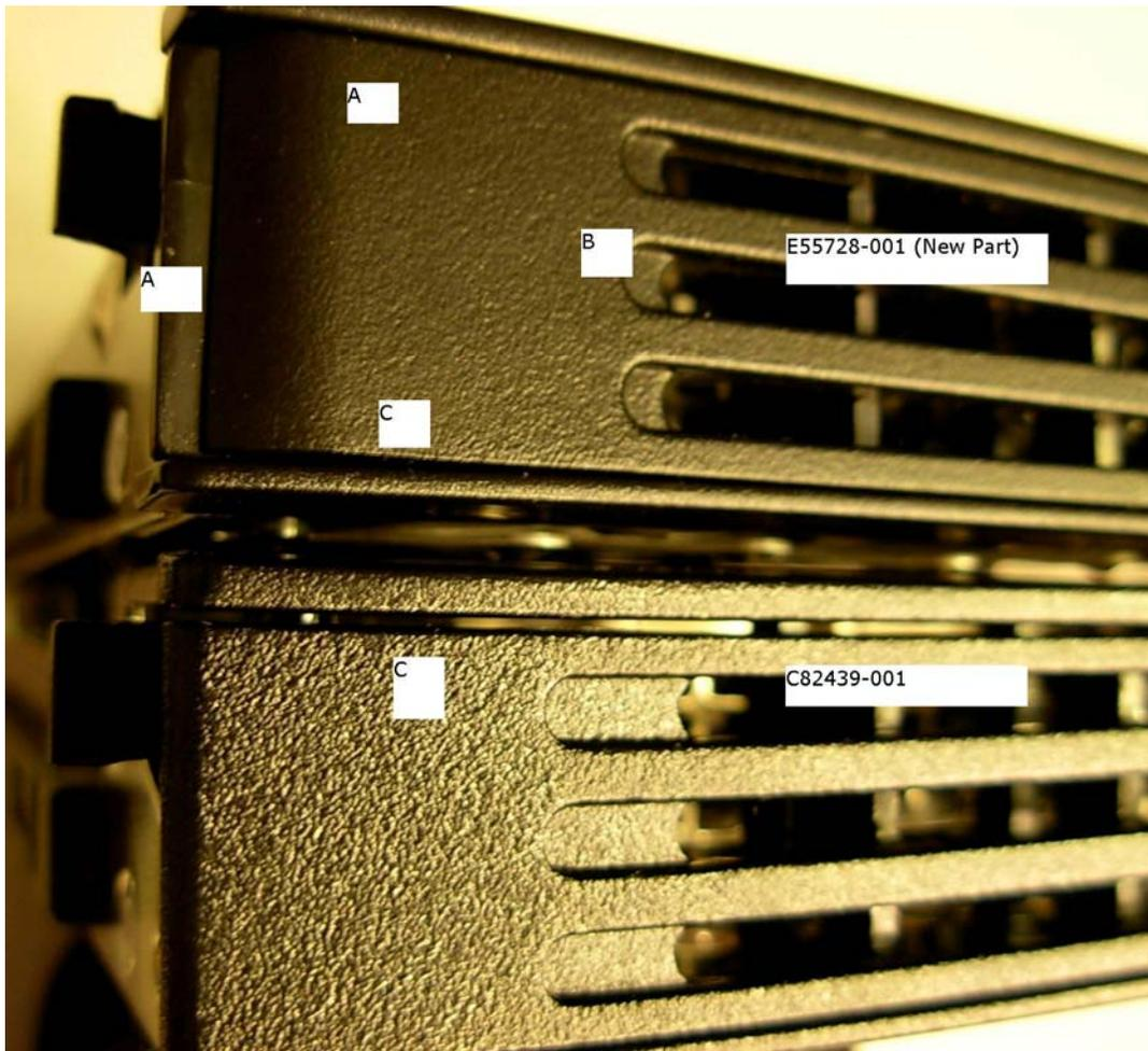
The top HDD carrier is the new vendor carrier as shown above. The new HDD part number is E55728-001 and looks nearly identical to the existing C82439-001 HDD carrier. The differences are outlined below.
