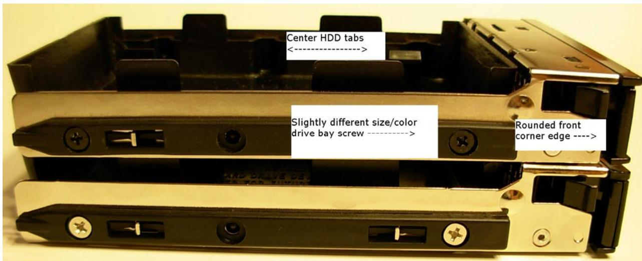
The top HDD carrier is the new carrier (E55728-001) with the changes highlighted. The new carrier includes a slightly different size/color drive bay screw. It includes the center HDD tabs on the drive baffle. These center HDD tabs are also referred to as snap features in the disposable air baffle. They have no impact to the functionality of the air baffle.
