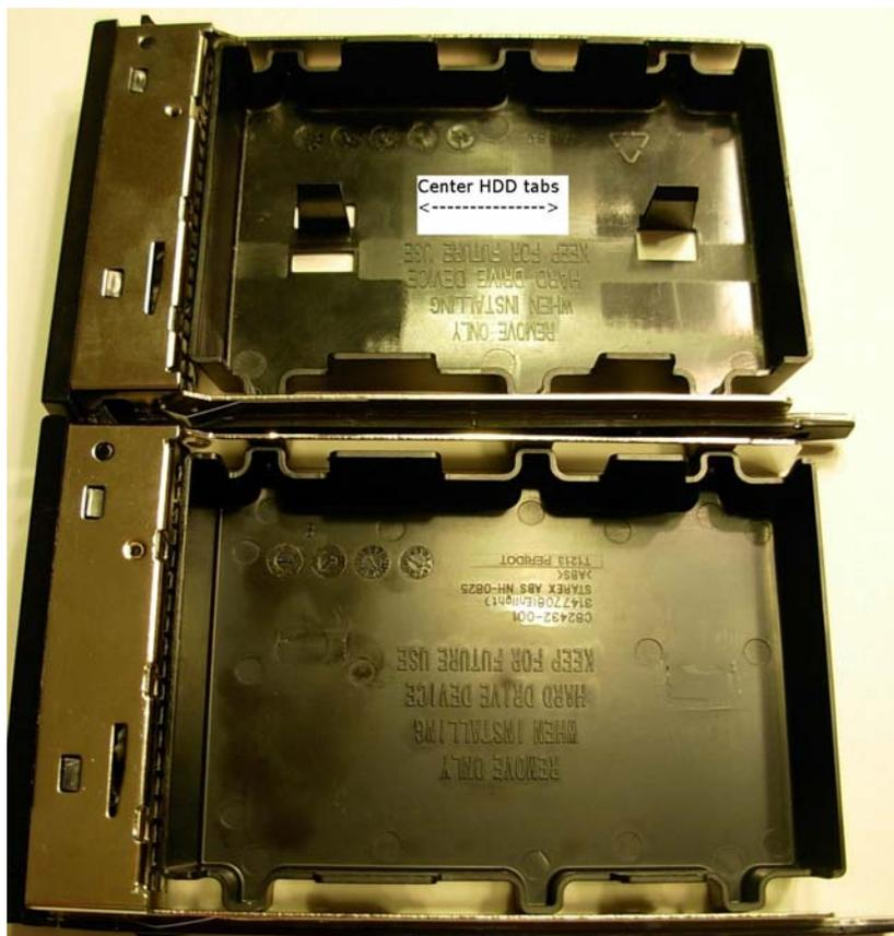
Other cosmetic differences are a slightly rounded front corner edge on the left side (A), a louvered indentation that does not extend as far to the left corner of the driver carrier (B), and a slightly smoother plastic texture on the bezel (C) as shown in the photograph below.
