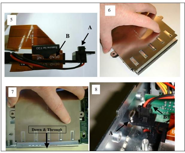
5. Power cable should plug into carrier opening (A) and be positioned as shown. The end of the Flex cable should route up through the slot in carrier (B) if pull-tab is present.
