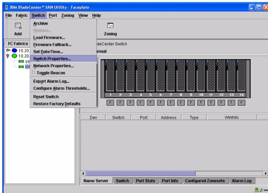
3. From the **Switch Properties—IBM BladeCenter SAN Utility** dialog box, verify that **R\_A\_TOV** is set to **10000** and **E\_D\_TOV** is set to **2000**. If the settings are not correct, proceed to [step 4](#). If the settings are correct, no changes need to be made; proceed to the next appropriate section.
