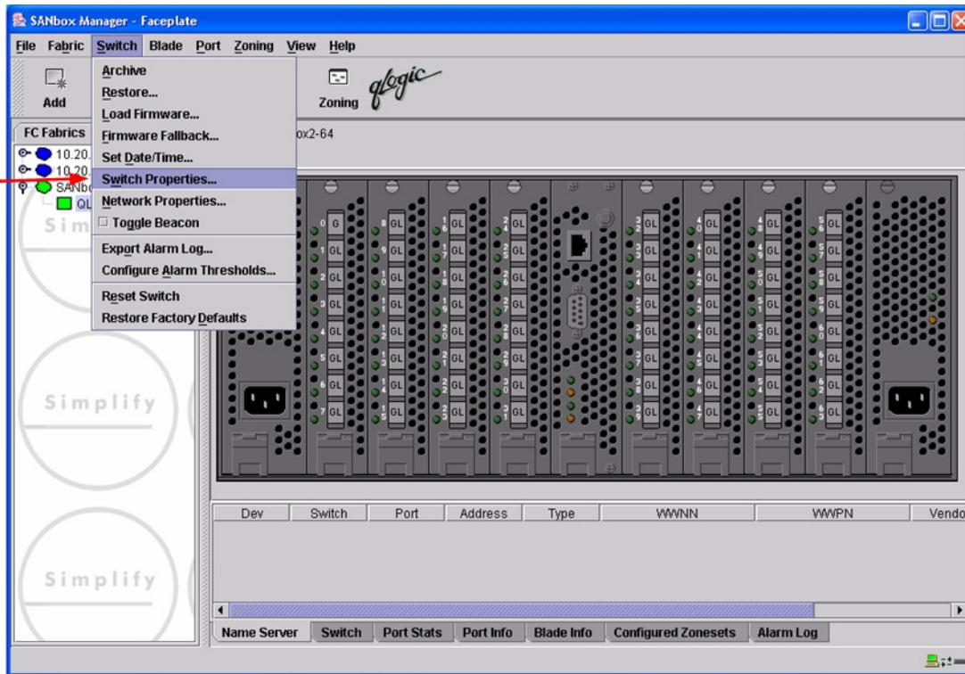
3. From the **Switch Properties—SANbox Manager** dialog box, verify that **R\_A\_TOV** is set to **10000** and **E\_D\_TOV** is set to **2000**. If the settings are not correct, proceed to [step 4](#). If the settings are correct, no changes need to be made; proceed to the next appropriate section.
