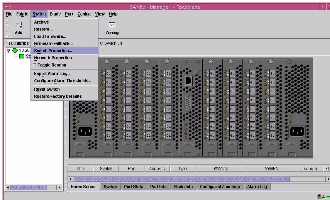
3. From the **Switch Properties—SANbox Manager** dialog box, verify that **R\_A\_TOV** is set to **10000** and **E\_D\_TOV** is set to **2000**. If the settings are not correct, proceed to [step 4](#). If the settings are correct, no changes need to be made; proceed to the next appropriate section.
