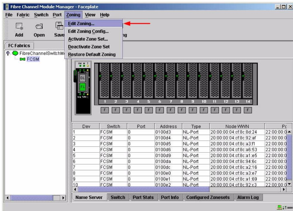
3. From the **Edit Zoning—Fibre Channel Module Manager** dialog box, compare the Zone Set and Zone names from each switch to ensure that none have the same name and the names conform to the standards for zone naming as discussed under “[Active Zone Set Names](#)” on page 23.
