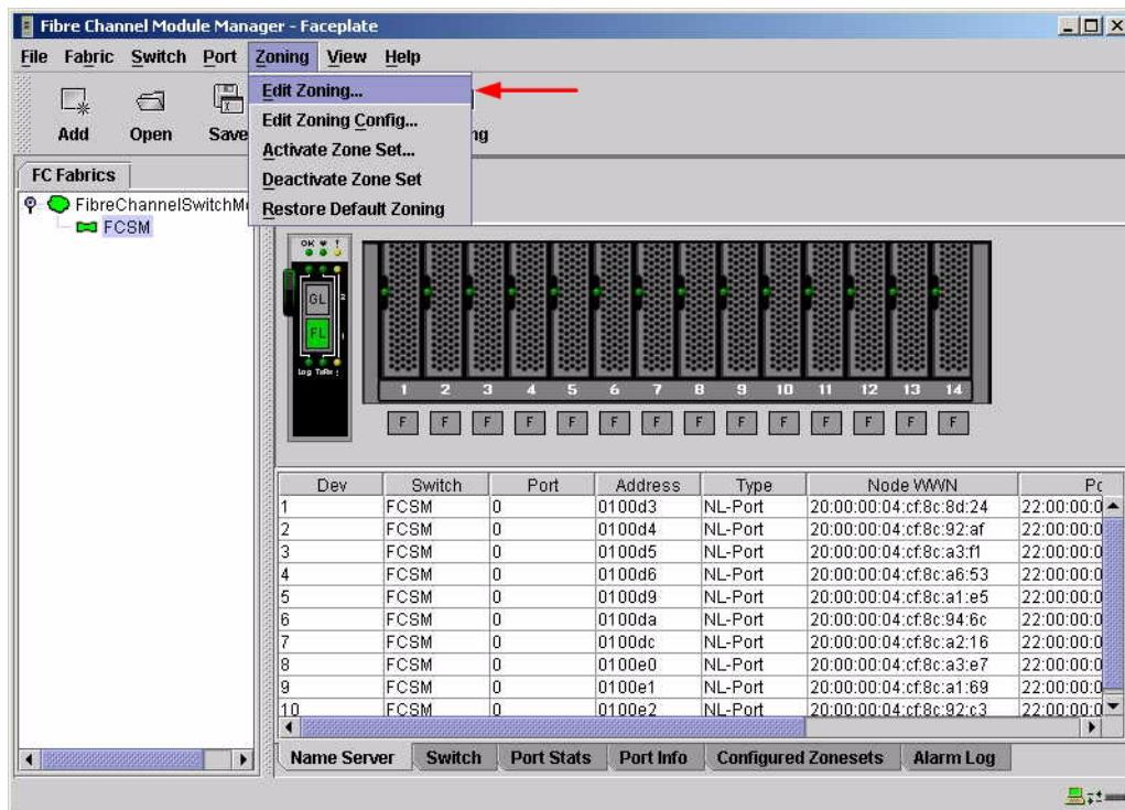
3. From the **Edit Zoning—Fibre Channel Module Manager** dialog box, compare the Zone Set and Zone names from each switch to ensure that none have the same name and the names conform to the standards for zone naming as discussed under “[Active Zone Set Names](#)” on page 131.
