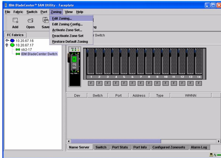
3. From the **Edit Zoning—IBM BladeCenter SAN Utility** dialog box, compare the Zone Set and Zone names from each switch to ensure that none have the same name and the names conform to the standards for zone naming as discussed under “[Active Zone Set Names](#)” on page 113.
