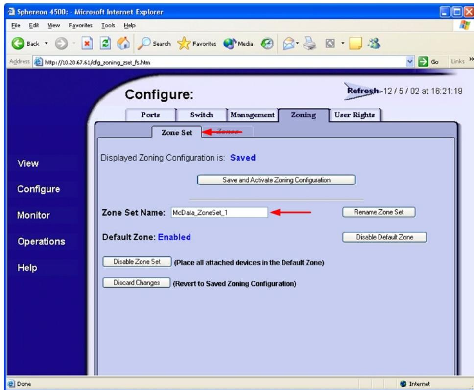
3. On the navigation panel, select **Configure**. The **Configure** dialog box displays. Select the **Zoning** tab, then select the **Zones** tab. Verify that the Zone names conform to the standards for zone naming as discussed under “[Active Zone Set Names](#)” on page 165.
