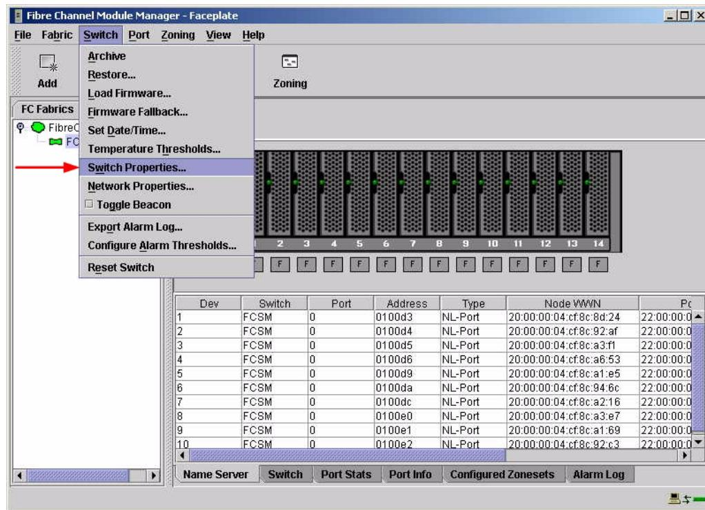
3. From the **Switch Properties—Fibre Channel Module Manager** dialog box, verify that **R\_A\_TOV** is set to **10000** and **E\_D\_TOV** is set to **2000**. If the settings are not correct, proceed to [step 4](#). If the settings are correct, no changes need to be made; proceed to the next appropriate section.
