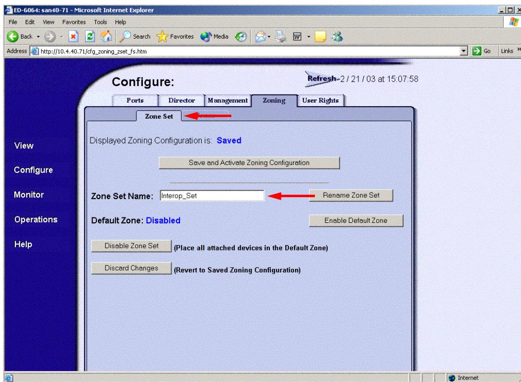
3. On the navigation panel, select **Configure**. The **Configure** dialog box displays. Select the **Zoning** tab, then select the **Zones** tab. Verify that the Zone names conform to the standards for zone naming as discussed under “[Active Zone Set Names](#)” on page 198.
