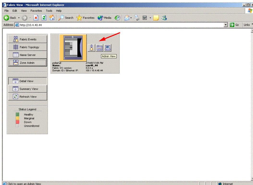
3. From the **Switch Admin for Brocade** dialog box, select the **Configure** tab. Verify that **R\_A\_TOV** is set to **10000** and **E\_D\_TOV** is set to **2000**. If the settings are not correct, do the following:
