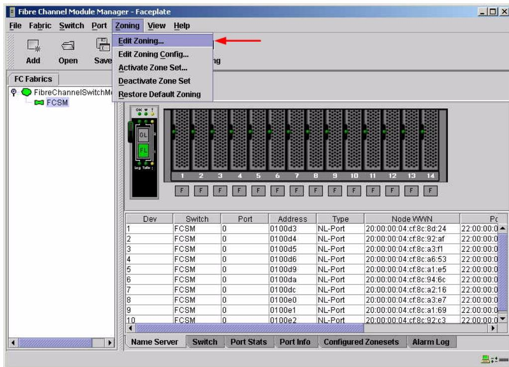
3. From the **Edit Zoning—Fibre Channel Module Manager** dialog box, compare the Zone Set and Zone names from each switch to ensure that none have the same name and the names conform to the standards for zone naming as discussed under “[Active Zone Set Names](#)” on page 165.
