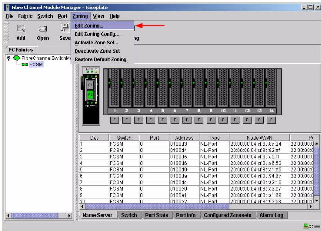
3. From the **Edit Zoning—Fibre Channel Module Manager** dialog box, compare the Zone Set and Zone names from each switch to ensure that none have the same name and the names conform to the standards for zone naming as discussed under “[Active Zone Set Names](#)” on page 233.
