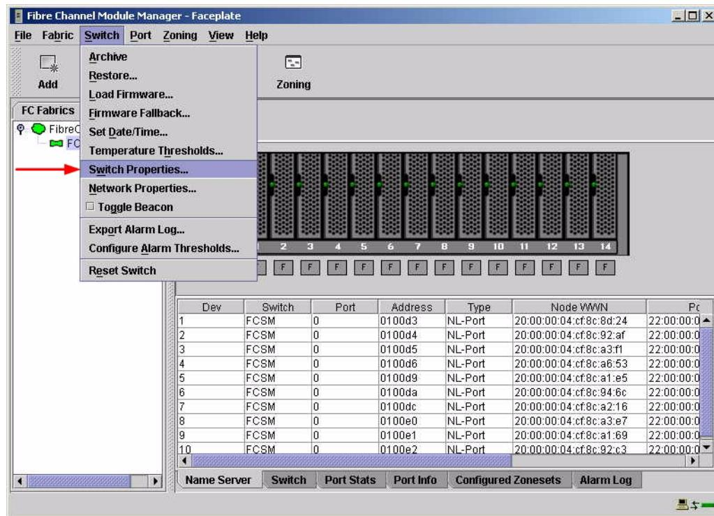
3. From the **Switch Properties—Fibre Channel Module Manager** dialog box, verify that **R\_A\_TOV** is set to **10000** and **E\_D\_TOV** is set to **2000**. If the settings are not correct, proceed to [step 4](#). If the settings are correct, no changes need to be made; proceed to the next appropriate section.
