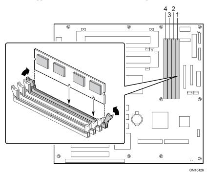
Figure 3. Installing DIMMs
