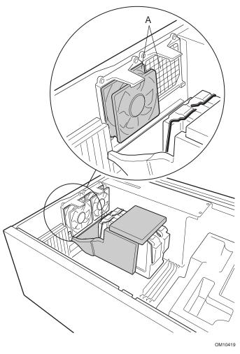
A. Fans Figure 5. Remove Auxiliary Fans
