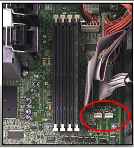
4. Plug both of the converter cables side labeled P1 into the connectors on the Server board labeled P20 and P21. Tuck cables away in order to maximize airflow.
