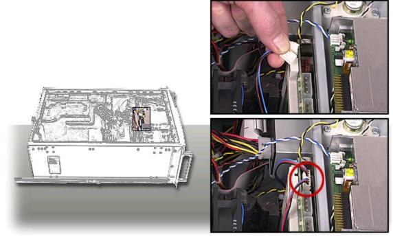
2. Remove the two fan connectors from the hot swap back plane.
