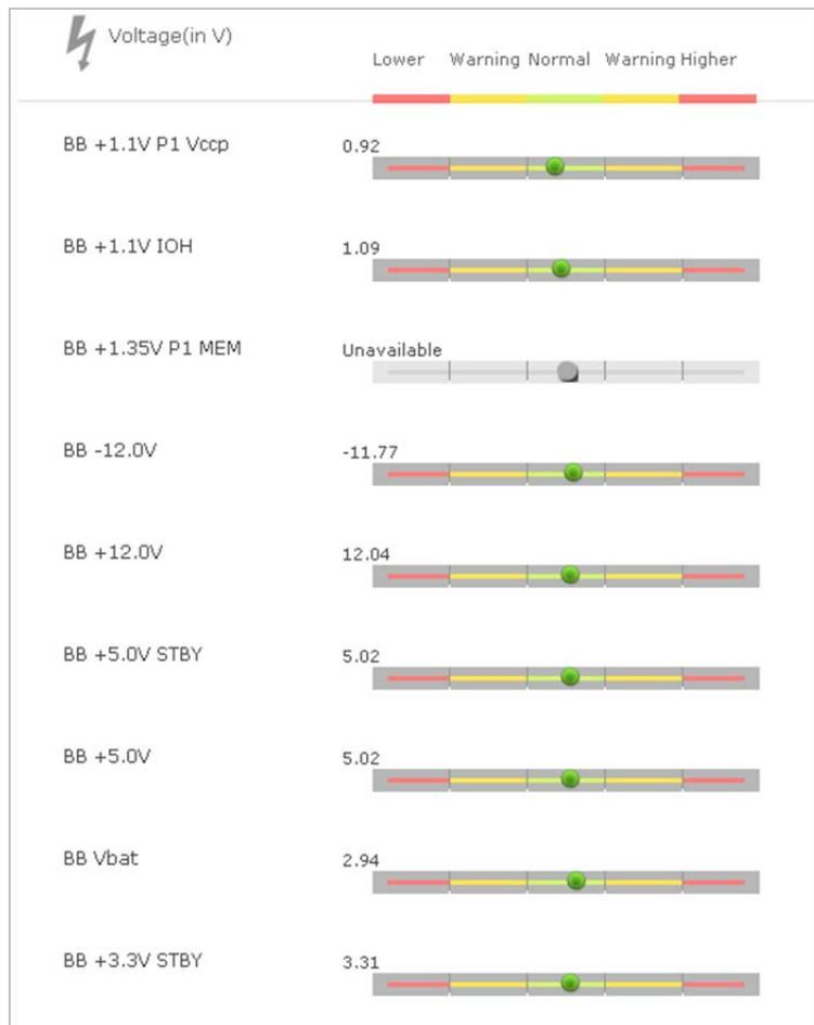
**Figure 4-11: Voltage Sensor Information**
