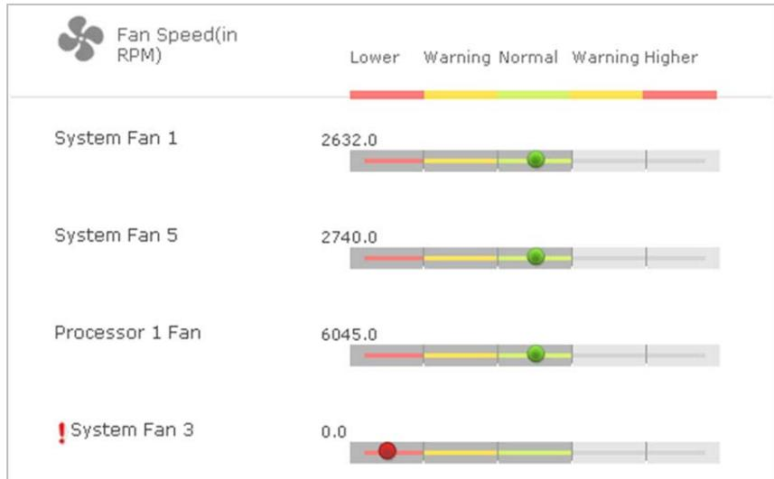
**Figure 4-10: Fan Speed Sensor Information**
