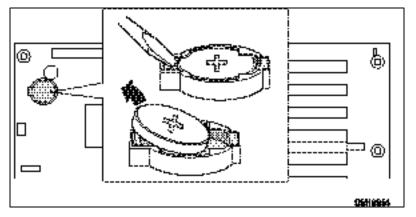
Figure 26. Replacing the Back up Battery
