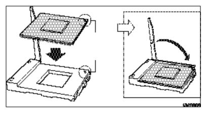
Figure 21. Insert the Processor
