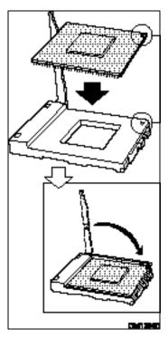
Figure 7. Inserting the Processor
