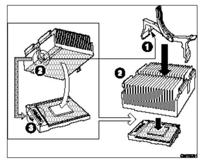
Figure 8. Attaching the Heat Sink and Retention Clip
