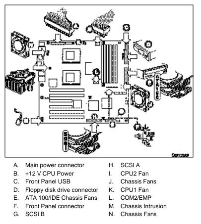
Figure 15. Making Connections to the Server Board
