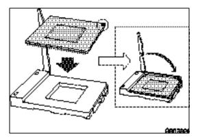
Figure 25. Installing a Terminator
