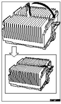
Figure 9. Locking the Heat Sink Retention Clip
