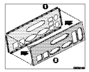
Figure 3. Attaching the Gasket to the I/O Shield
