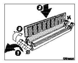
Figure 12. Installing Memory
