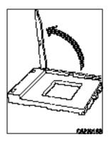
Figure 20. Raise the Locking Bar
