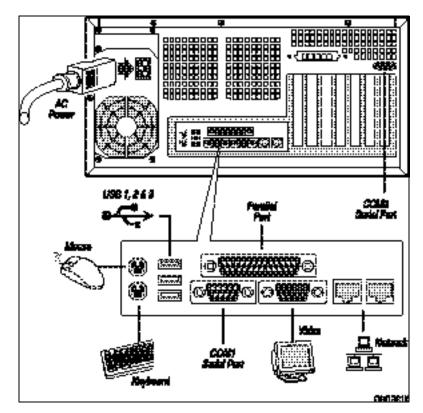
Figure 19. Making Back Panel Connections
