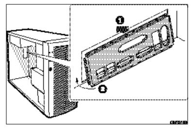
Figure 5. Installing the I/O Shield
