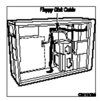
Figure 17. Routing the Floppy and USB Cables
