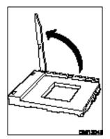
Figure 6. Lifting the Locking Bar
