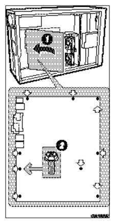
Figure 14. Placing the Server Board in the Chassis
