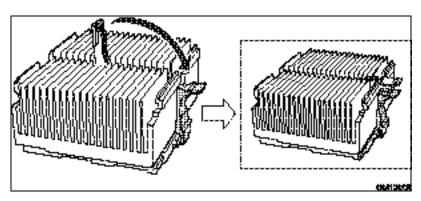
Figure 23. Lock the Heat Sink Retention Clip
