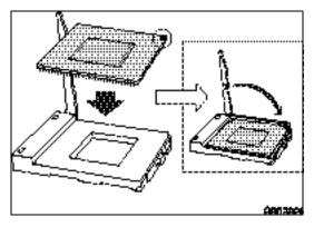
Figure 11. Installing a Terminator
