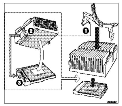
Figure 22. Attach the Heat Sink and Retention Clip
