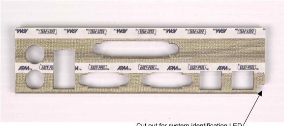
Cut out for system identification LED
