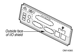
Figure 4. Attaching the Label to the I/O Shield
