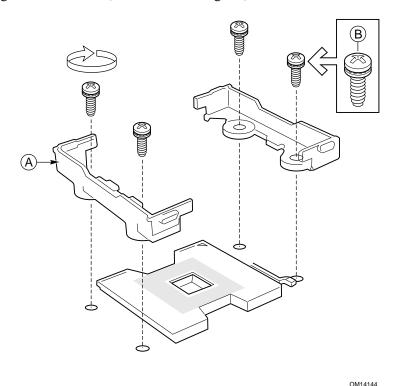
Figure 19. Installing the Processor Retention Brackets
