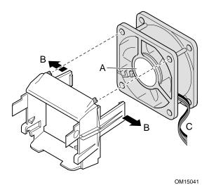
Figure 15. Attaching the Wind Tunnel Fan
