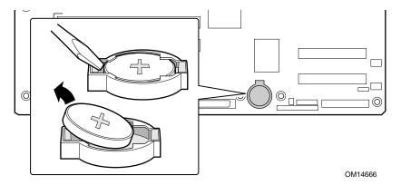
Figure 28. Replacing the Backup Battery
