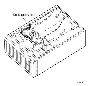
Figure 10. Routing the SCSI and Floppy Drive Cable
