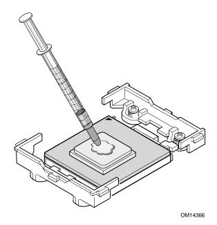
Figure 23. Applying Thermal Grease
