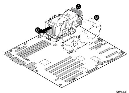
Figure 18. Processor and Wind Tunnel Installed
