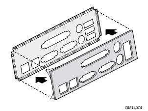
Figure 3. Attaching the Gasket to the I/O Shield
