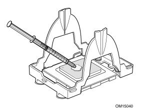
Figure 13. Applying Thermal Grease
