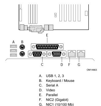
Figure 2. Back Panel Connectors
