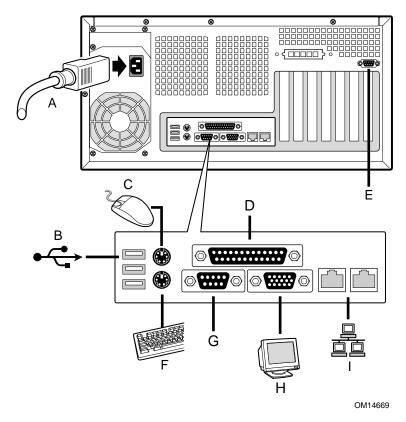
Figure 27. Making Back Panel Connections
