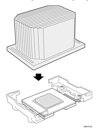
Figure 24. Installing the Heat Sink
