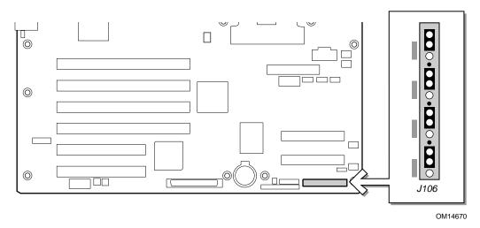
Figure 32. Configuration Jumper Location
