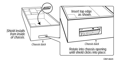
Figure 5. Installing the I/O Shield
