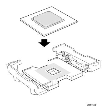
Figure 21. Installing Processors
