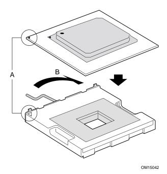
Figure 11. Opening Socket Lever and Attaching Processor
