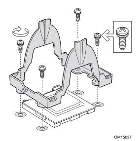
Figure 12. Attaching Retention Mechanism
