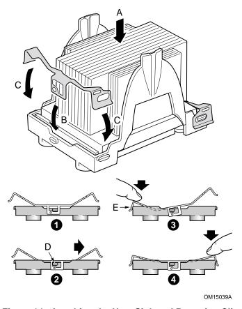
Figure 14. Attaching the Heat Sink and Retention Clip
