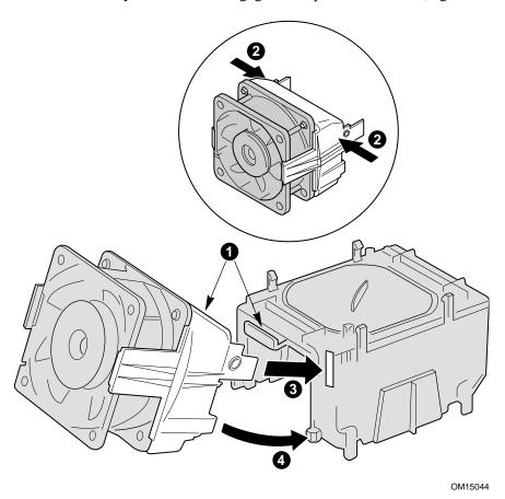
Figure 16. Attaching the Heat Sink Fan to the Top of the PWT
