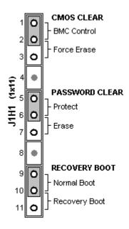
Figure 31. CMOS Recovery Jumper
