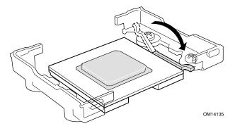
Figure 22. Lower Locking Bar
