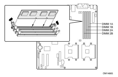
Figure 26. Installing Memory
