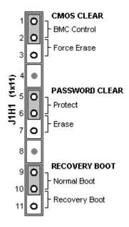
Figure 30. Password Recovery Jumper
