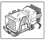
When installing only one processor, there is no need to install the wind tunnel assembly over the second processor location. Use the wind tunnel assembly over a CPU socket only when a CPU is installed.
