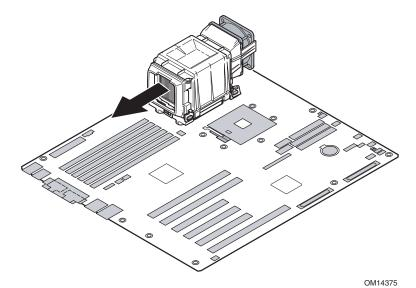
Figure 15. Processor Wind Tunnel Air Flow
