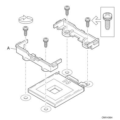
Figure 27. Installing the Retention Brackets
