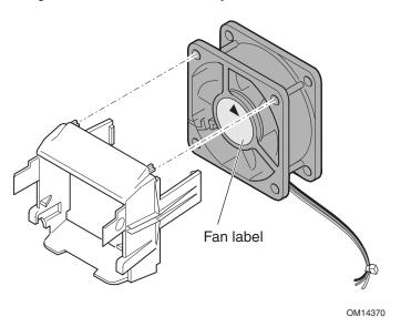
Figure 17. Attaching the Heat Sink Fan to the Air Intake Assembly
