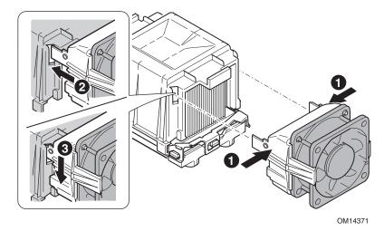
Figure 34. Attaching the Wind Tunnel Intake and Exhaust
