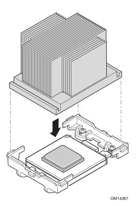
Figure 13. Aligning the Heat Sink
