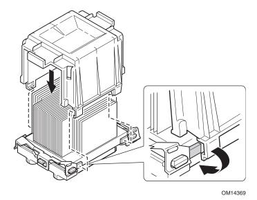
Figure 16. Attaching the Wind Tunnel Assembly
