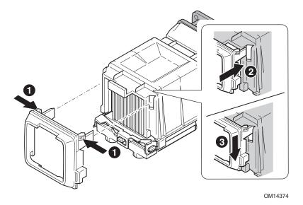
Figure 35. Attaching the Wind Tunnel Intake and Exhaust
