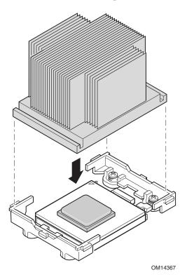
Figure 30. Aligning the Heat Sink
