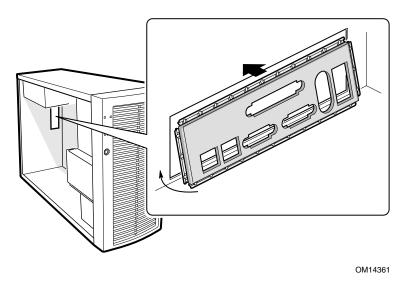
Figure 5. Installing the I/O Shield
