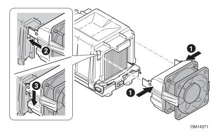
Figure 18. Attaching the Wind Tunnel Intake and Exhaust
