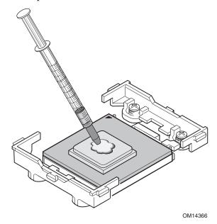
Figure 29. Applying Thermal Grease
