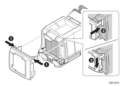
Figure 19. Attaching the Wind Tunnel Intake and Exhaust
