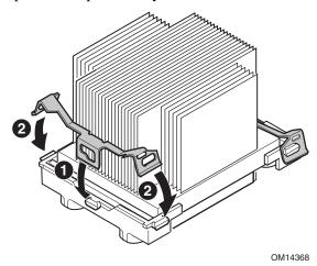
Figure 31. Attaching the Heat Sink and Retention Clip
