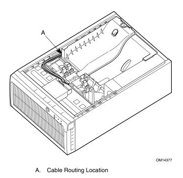
Figure 23. Routing the Floppy and ICMB Cables
