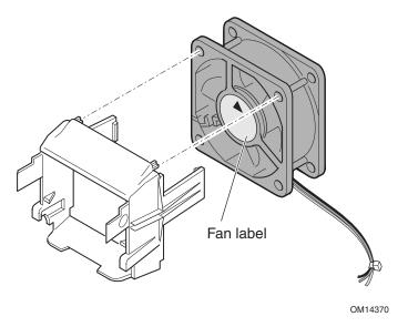
Figure 33. Attaching the Heat Sink Fan to the Air Intake Assembly
