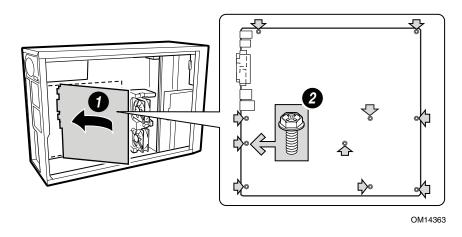
Figure 9. Placing the Server Board in the Chassis
