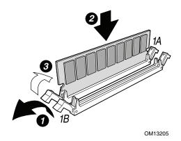
Figure 26. Installing Memory
