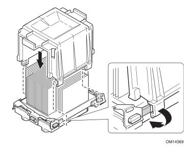
Figure 32. Attaching the Wind Tunnel Assembly
