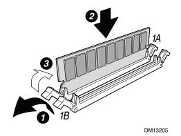
Figure 7. Installing Memory
