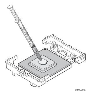
Figure 12. Applying Thermal Grease
