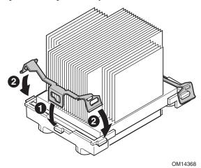
Figure 14. Attaching the Heat Sink and Retention Clip
