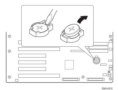
Figure 36. Replacing the Back up Battery
