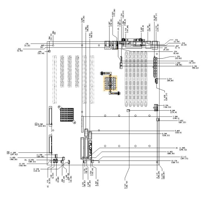
Figure 18. SHG2 Baseboard Mechanical Diagram 2
