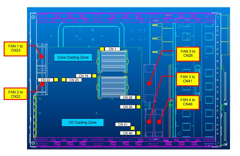
Figure 12. SHG2 System Redundant Cooling Fan Support
