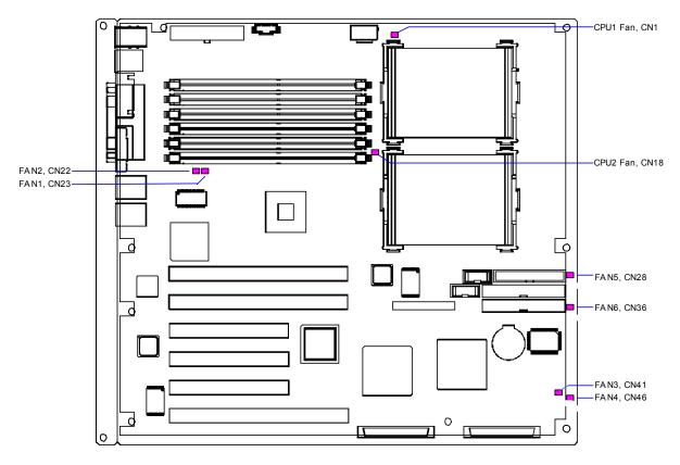
Figure 11. SHG2 Board Fan Connector Locations
