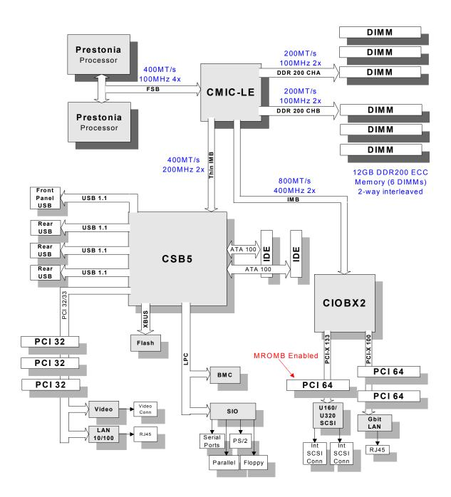
Figure 1. Intel<sup>®</sup> SHG2 Server Board
