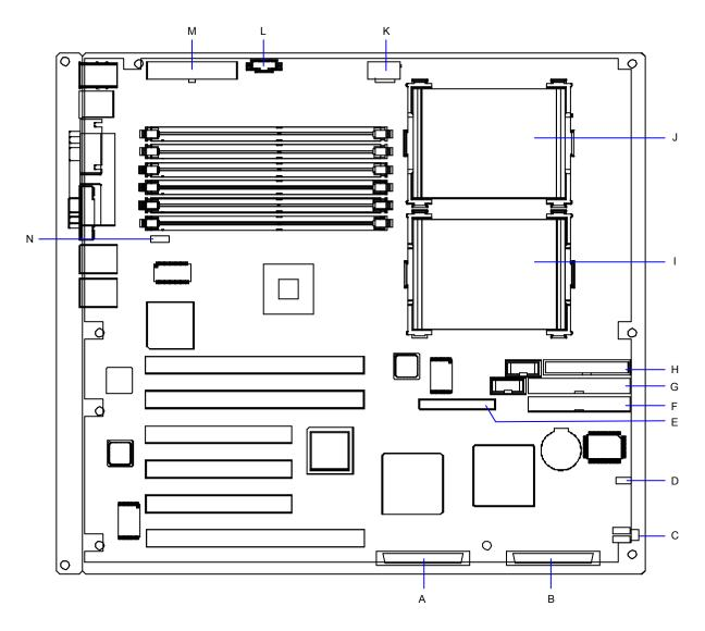
Figure 10. SHG2 Baseboard Connector Identification and Locations
