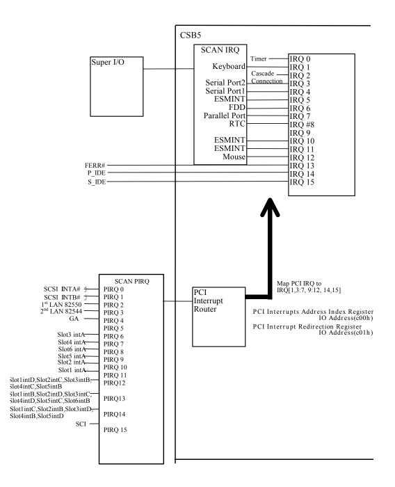
Figure 4. SHG2 Interrupt Routing (PIC Mode)
