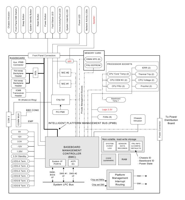
Figure 7. SHG2 Sahalee BMC Block Diagram
