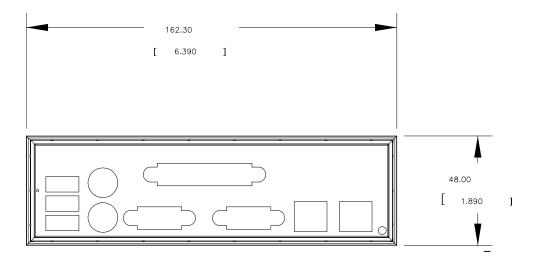
Figure 14. SHG2 I/O Panel Connector Location Dimensions
