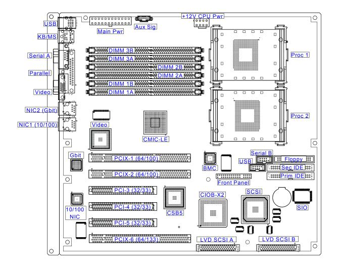
Figure 2. SHG2 Server Board Placement Diagram
