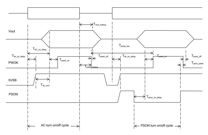
Figure 16. Turn On/Off Timing
