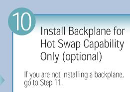
If you are installing an optional backplane, go to the backplane kit documentation for instructions on installing the backplane, air baffle and cabling.
