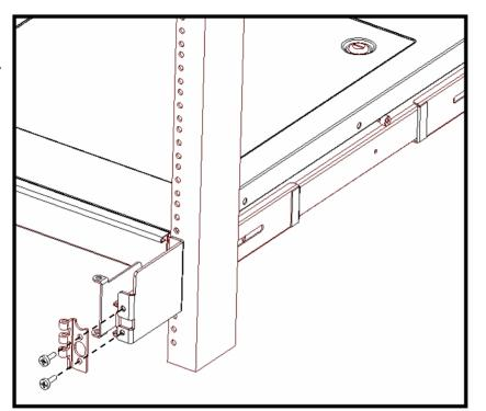
Assemble the Cable Carrier attachment bracket to the Rack Extension Bracket with two #10-32 screws from the Cable Carrier Kit.
