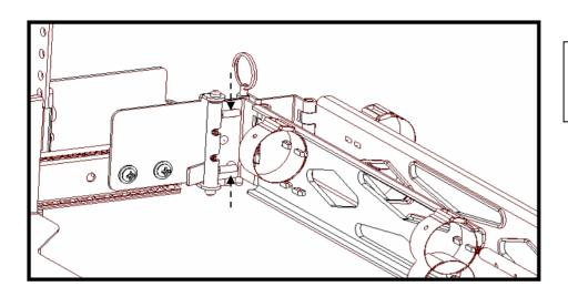
Depress the spring loaded pins to snap the front arm of the Cable Carrier to the Rail Kit Attachment Bracket.
