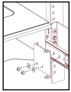
Attach the Rail Kit Attachment Bracket to the inner member of the chassis rail kit using the two ¼ inch long pan head machine screws and washers.
