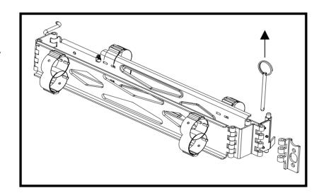
Pull the pin from the Cable Carrier assembly as shown and remove the attachment bracket.
