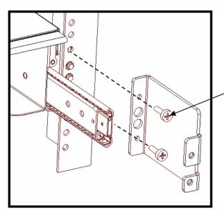
Remove the #10-32 screws from the rear attachment points of the rail kit as shown and use them to install the Rack Extension Bracket.
