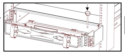
Install the Cable Carrier assembly as shown to the attachment bracket with the pin removed in Step # 4.
