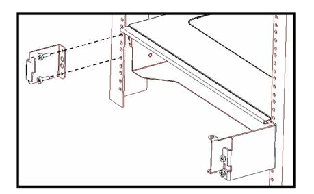
Remove the #10-32 screws from the rear attachment points of the rail kit as shown and use them to install the Cable Carrier Arm Stop Bracket.
