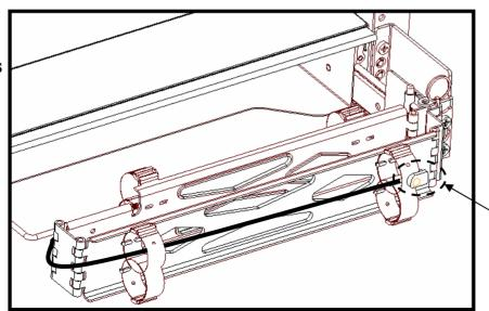
Locate Rear Status Indicator LED as shown attached to the velcro strap so that the LED is visible from the rear of the unit.
