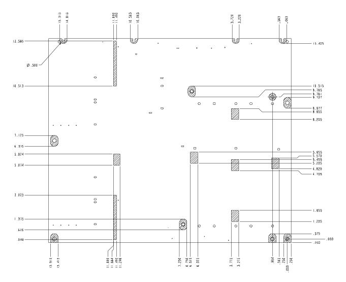
Figure 23. Secondary Side Surface Keep-outs
