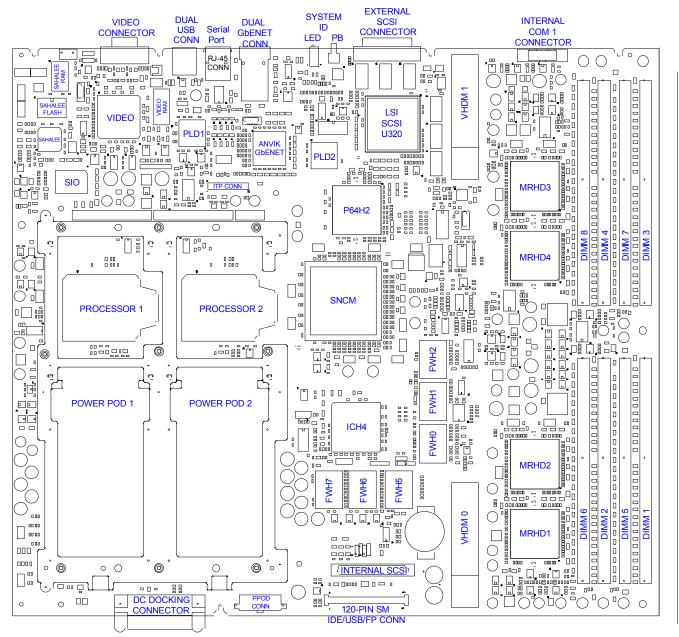
Figure 3. Mainboard Component Location (Primary Side)
