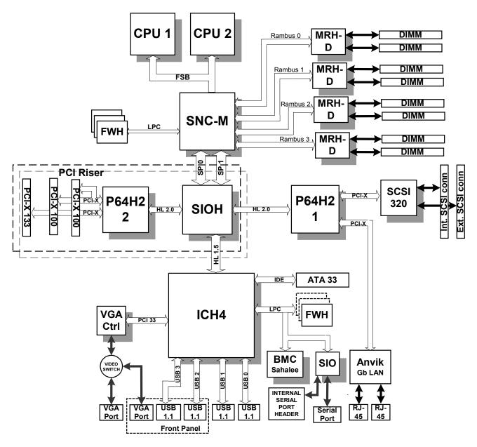
Figure 2. Mainboard Block Diagram
