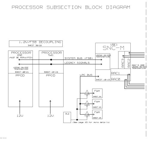
Figure 4. Processor Subsection Block Diagram
