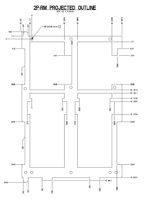
Figure 25. Processor Retention Mechanism
