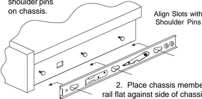
2. Place chassis member rail flat against side of chassis and move forward to allow shoulder pins to locate in small slots of keyholes.
