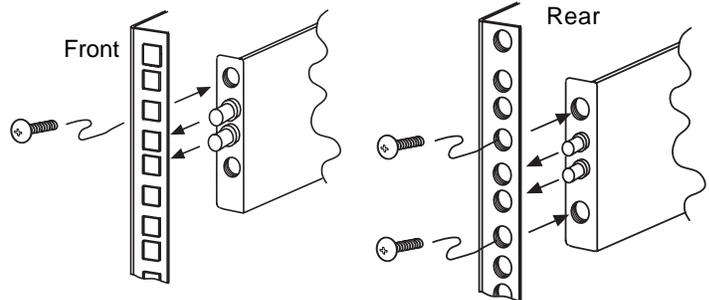
5. Install two flange head screws into rear cabinet rail in location shown. Tighten all screws completely.
