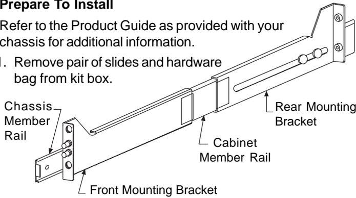
2. Hold cabinet member rail and chassis member rail of slide and fully extend slide to the open and locked position.
