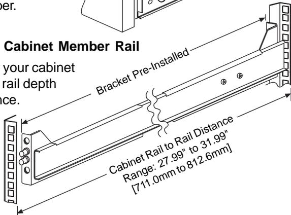
2. Hold the cabinet member rail up to the vertical columns of the rack cabinet with the outside faces of the flanges positioned inside the front and rear column.
