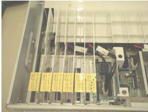
Figure 94. Locating the CPU1 / CPU2 MVR Connection
