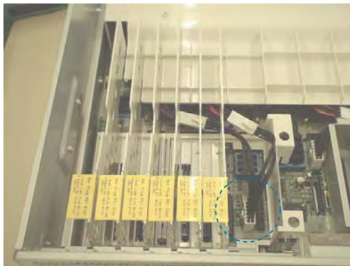
Figure 82. Locating the CPU1 / CPU2 MVR Connection
