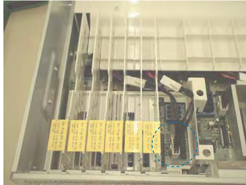
Figure 73. Locating the CPU1 / CPU2 MVR Connection
