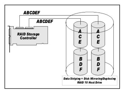
Figure 1-6. RAID 10 - Combination of RAID 1 and RAID 0
