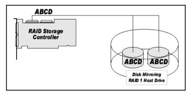
Figure 1-3. RAID 1 - Disk Duplexing
