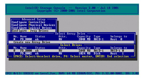
Figure 57. Create New Array Drive
