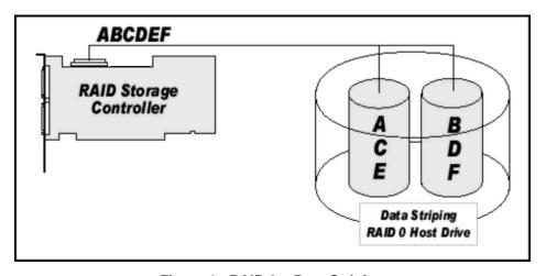
Figure 1. RAID 0 - Data Striping
