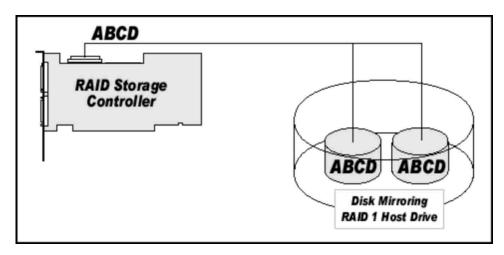
Figure 2. RAID 1 - Disk Mirroring
