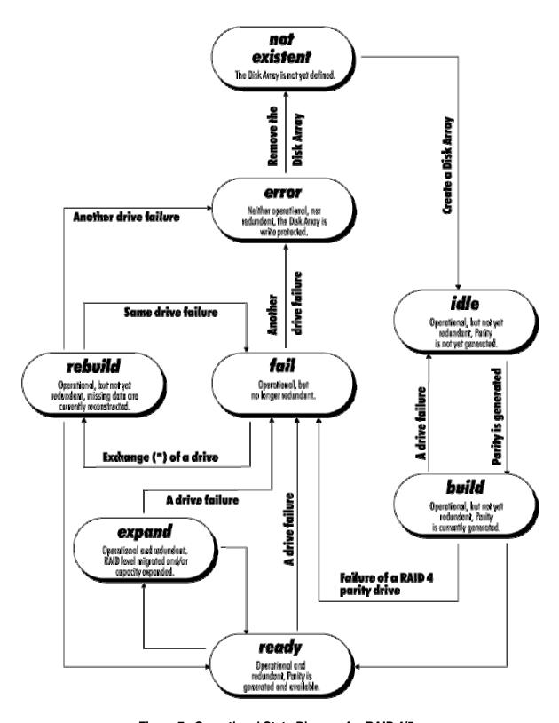
Figure 7. Operational State Diagram for RAID 4/5
