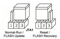
Figure 6. Jumper Positions for FLASH Update and Recovery
