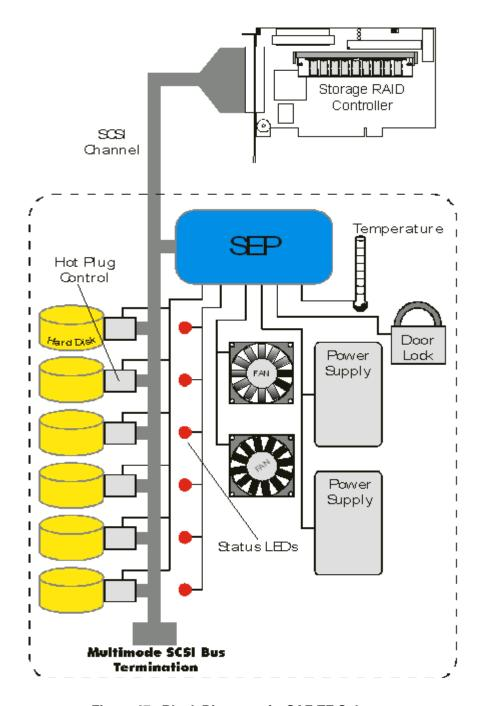
Figure 47. Block Diagram of a SAF-TE Subsystem
