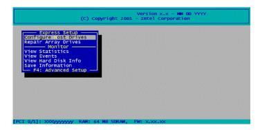
5. Select "Create New Host Drive." StorCon displays a list of "free" hard disk drives. These are drives that do not belong to a logical host drive and can be used for new host drives.
