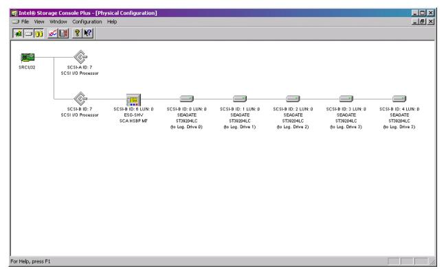
Figure 79. Example of a Physical Configuration and the Controller Settings
