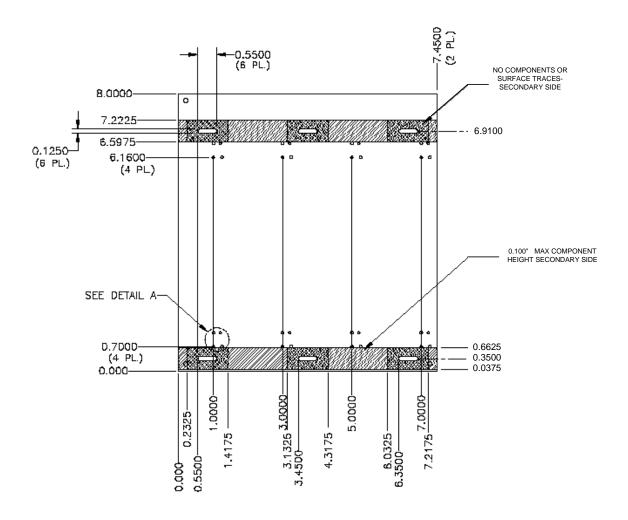
Figure 4-3. Mechanical Specifications
