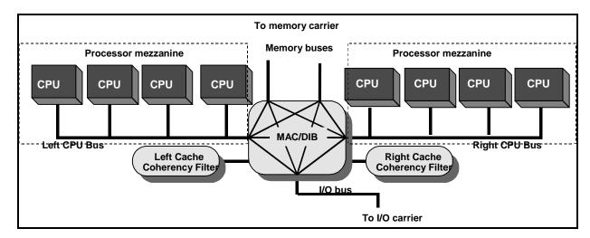
Figure 3-1: Profusion\* Carrier Block Diagram
