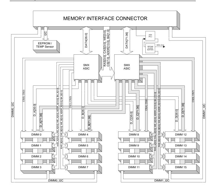
Figure 5-1: SRPL8 Memory Carrier Block Diagram
