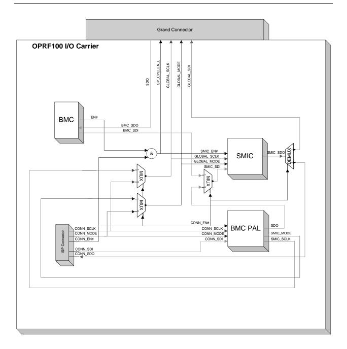
Figure 2-8: In-System Programming of Onboard PLDs
