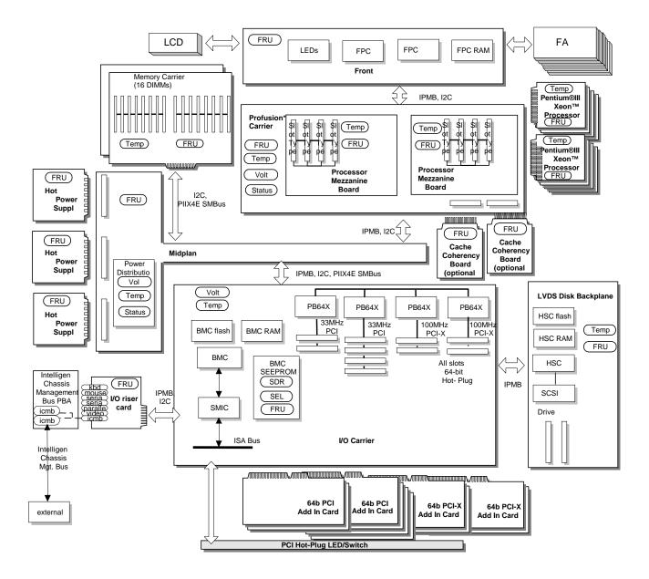
Figure 3-4: Profusion\* Carrier System Management Logic
