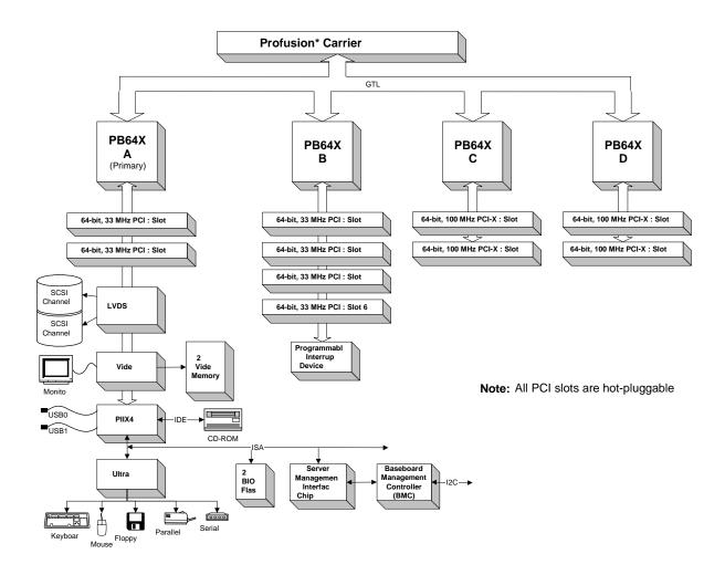
Figure 2-1: I/O Carrier Block Diagram
