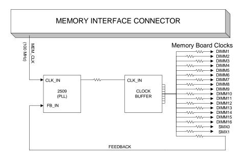
Figure 5-2: SRPL8 Memory Carrier Clock Distribution Diagram
