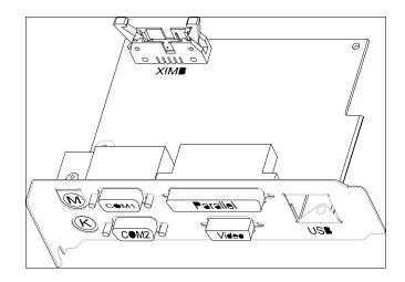
Figure 2-14: A450NX I/O Riser Board Mechanical Diagram
