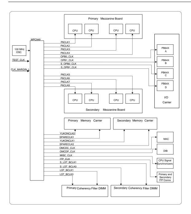
Figure 3-3: Profusion\* Carrier Clock Distribution
