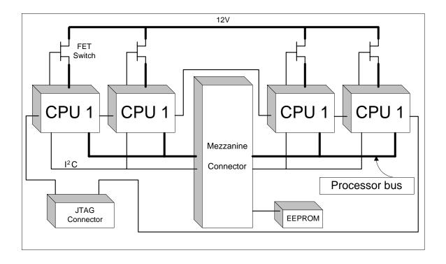
Figure 4-1. SRPL8 Processor Mezzanine Board Block Diagram
