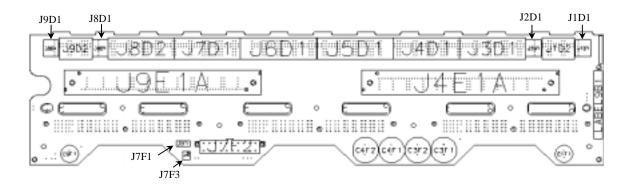
Figure 6-2: Placement Diagram (Secondary Side)
