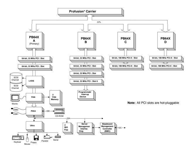
Figure 2-4: I/O Carrier Block Diagram
