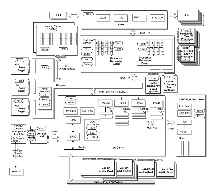
Figure 1-1: SRPL8 Boardset Block Diagram
