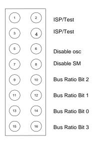
Figure 3-5: J6A1 Jumper Connector Pinout
