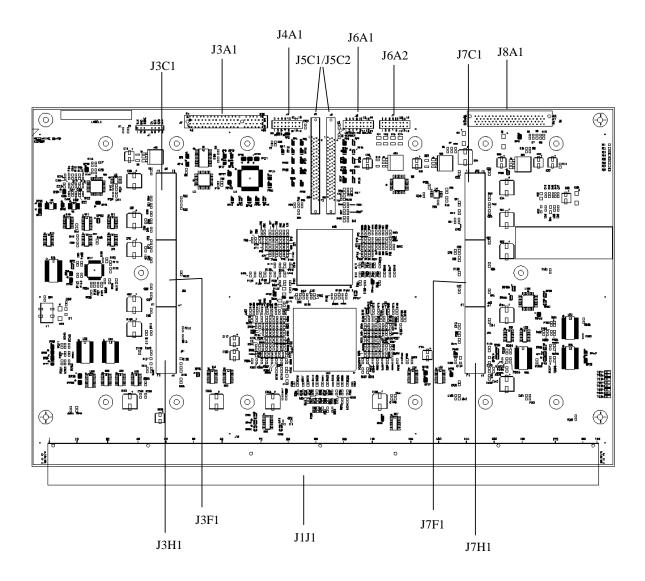
Figure 3-2: Profusion\* Carrier Layout
