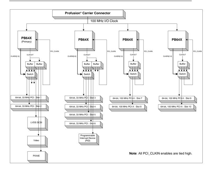
Figure 2-11: I/O Carrier Clocking Architecture
