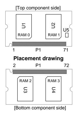
Figure 7-2: Cache Coherency Board
