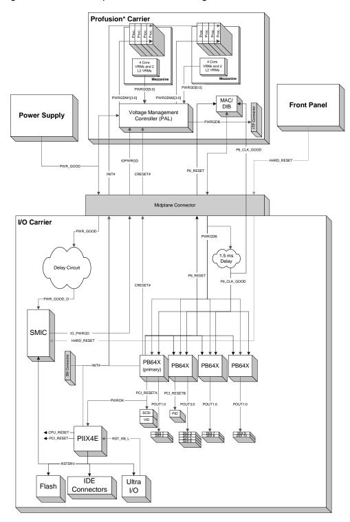
Figure 2-12: Reset Diagram
