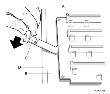
Figure 45. Separating the Profusion Carrier and Processor Mezzanine Boards
