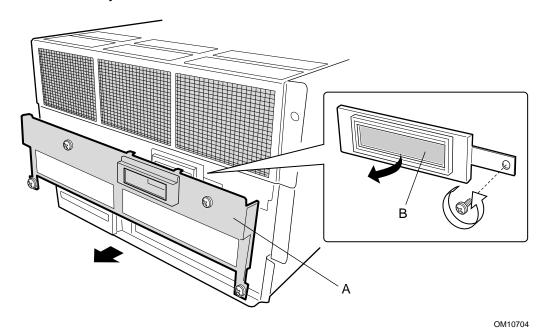
Figure 27. Removing the LCD Module
