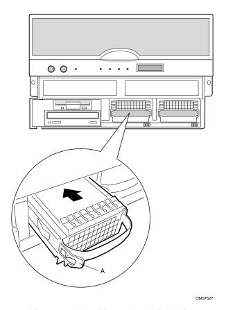
Figure 18. Installing a Hard Disk Drive
