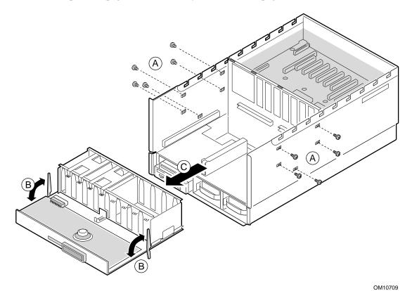
Figure 28. Removing the Profusion Carrier Tray
