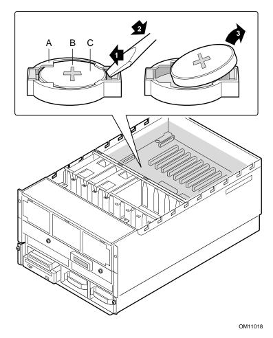
Figure 54. Replacing the Lithium Battery
