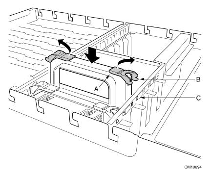
Figure 53. Installing a Termination Board Assembly
