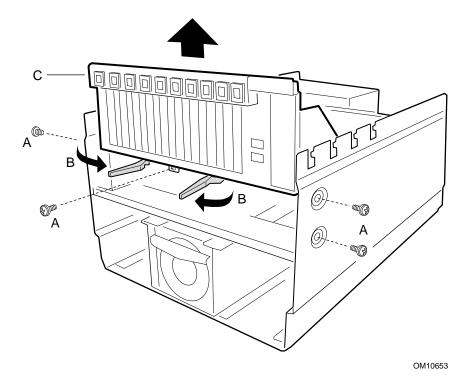
Figure 34. Removing the I/O Tray
