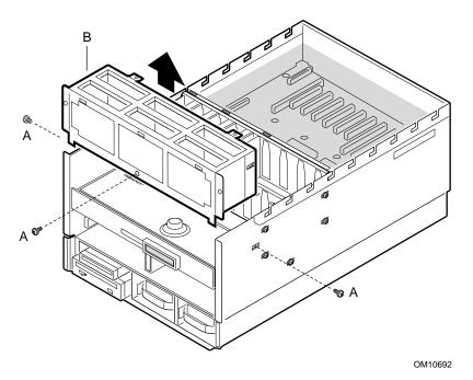
Figure 26. Removing the Fan Housing
