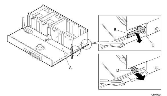
Figure 44. Removing the Processor Retention Bracket
