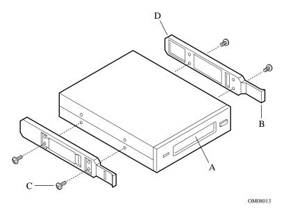
Figure 41. Snap-in Plastic Slide Rails
