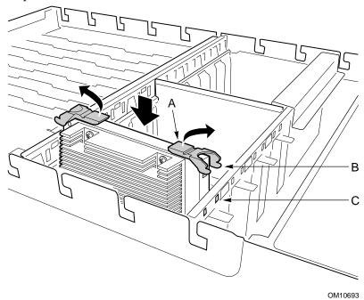
Figure 52. Installing a Processor
