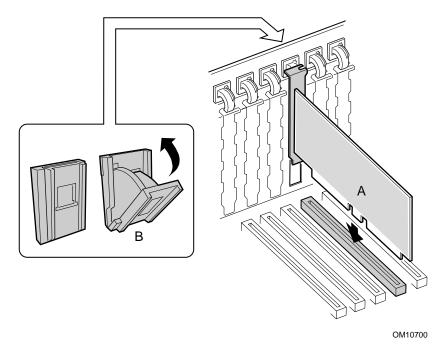
Figure 31. Installing an Add-in Board
