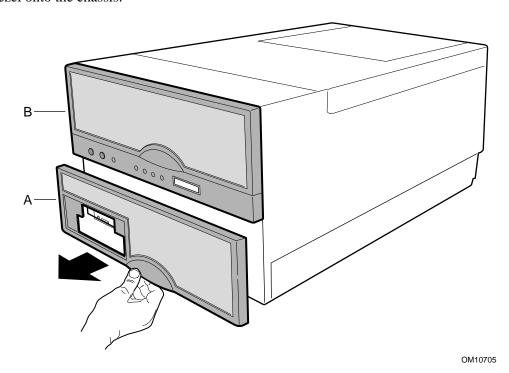
Figure 20. Removing the Front Bezels
