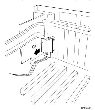
Figure 35. Removing the ICMB Board
