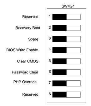
Figure 57. I/O Carrier Configuration Switches
