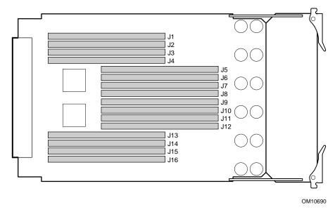
Figure 49. DIMMs Slot Layout
