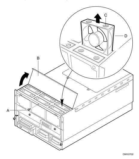
Figure 15. Removing/Hot-swapping a Fan
