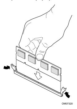
Figure 50. Installing DIMMs
