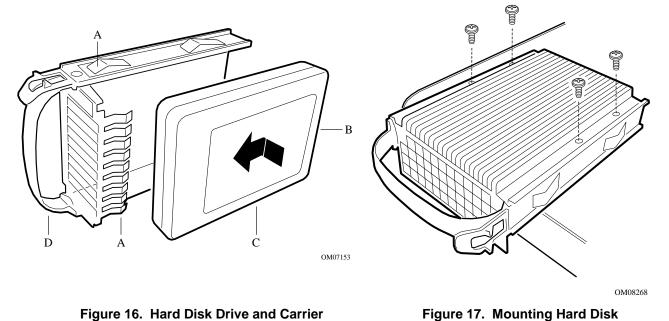
Figure 16. Hard Disk Drive and Carrier
