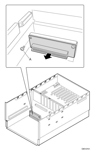
Figure 38. Peripheral Bay Blind Mate Board
