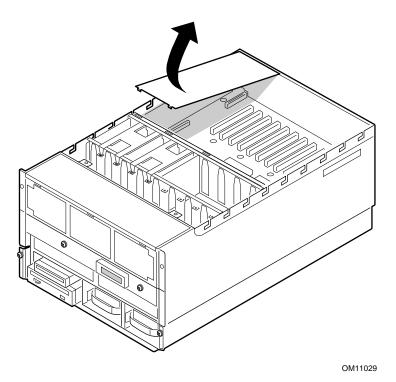
Figure 24. Removing the 240 VA Protective Cover
