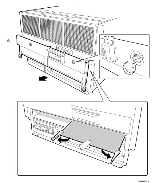
Figure 25. Removing the Memory Module Cover and Memory Module
