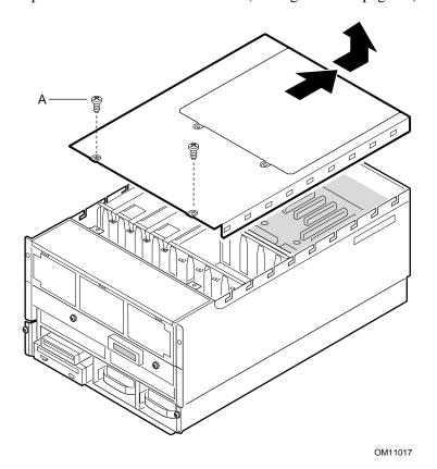
Figure 23. Removing the Top Cover
