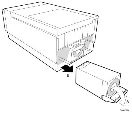
Figure 19. Removing a Power Supply
