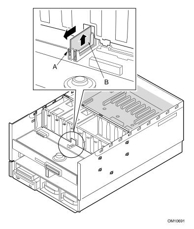
Figure 43. Removing the Cache Coherency Filters
