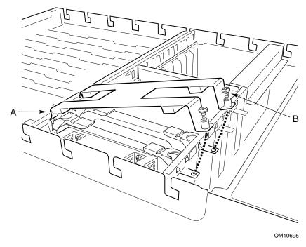
Figure 51. Removing a Processor Holddown
