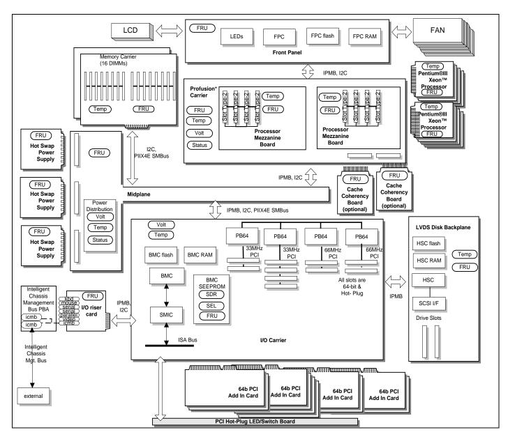
Figure 3-4: Profusion\* Carrier System Management Logic
