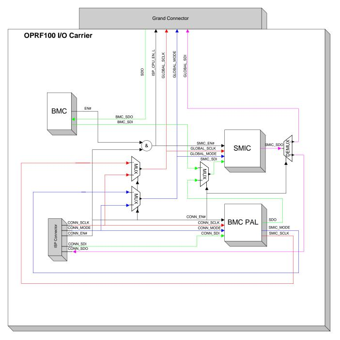
Figure 2-8: In-system-Programming of Onboard PLDs
