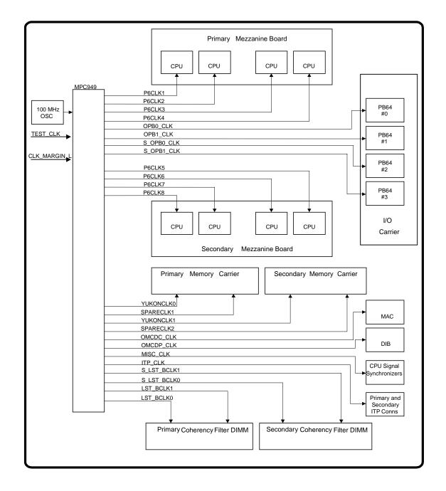
Figure 3-3: Profusion\* Carrier Clock Distribution
