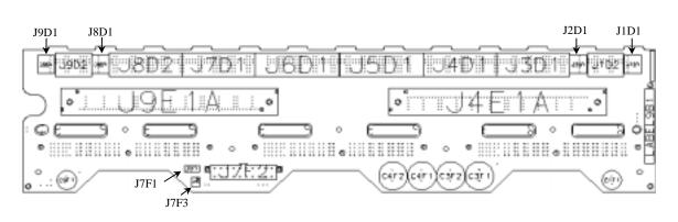
Figure 6-2: Placement Diagram (secondary side)
