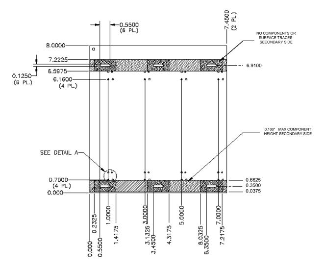
Figure 4-3: Mechanical Specifications
