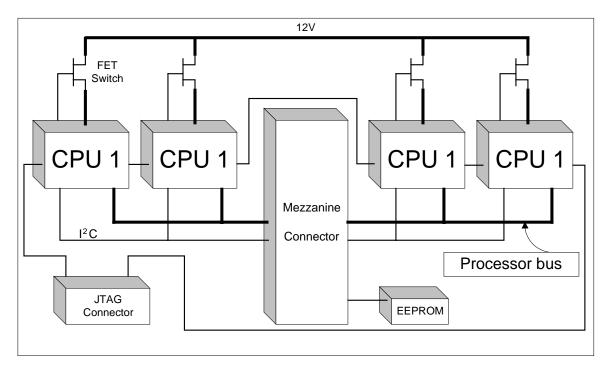
Figure 4-1: SRPM8 Processor Mezzanine Board Block Diagram
