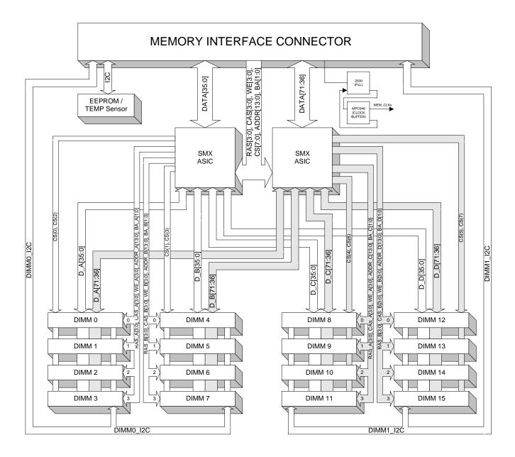
Figure 5-1: OCPRF100 Memory Carrier Block Diagram
