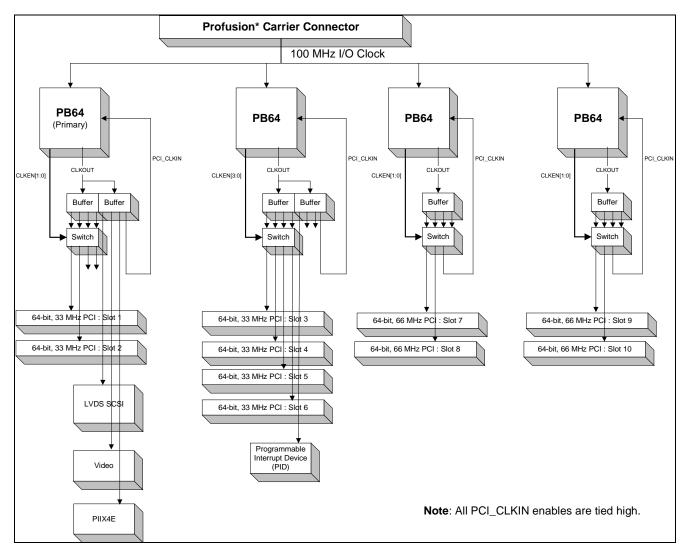
Figure 2-11: I/O Carrier Clocking Architecture
