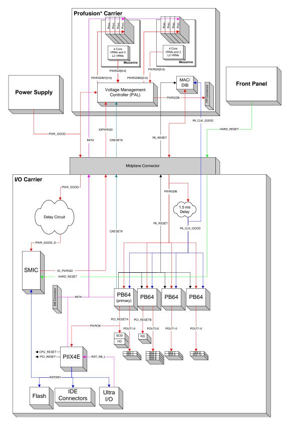
Figure 2-12: Reset Diagram
