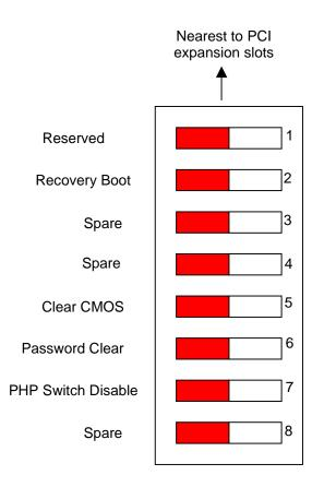
Figure 2-10: I/O Carrier Configuration Switches
