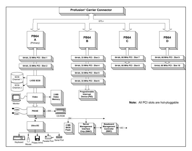
Figure 2-1: I/O Carrier Block Diagram
