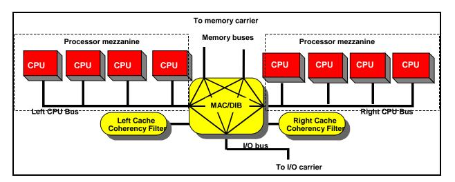
Figure 3-1: Profusion\* Carrier Block Diagram
