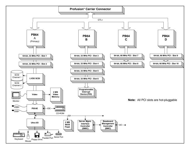
Figure 2-4: I/O Carrier Block Diagram
