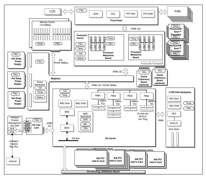
Figure 1-1: SRPM8 Board Set Block Diagram
