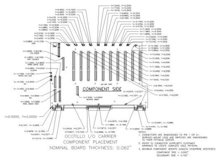
Figure 2-13: I/O Carrier Mechanical Diagram
