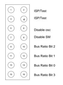
Figure 3-5: J6A1 Jumper Connector Pinout
