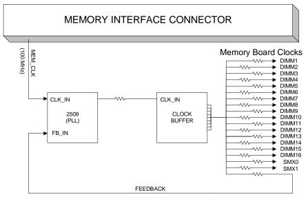
Figure 5-2: OCPRF100 Memory Carrier Clock Distribution Diagram
