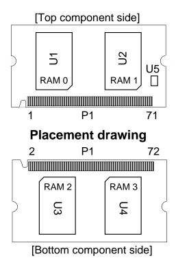
Figure 7-2: Cache Coherency Board
