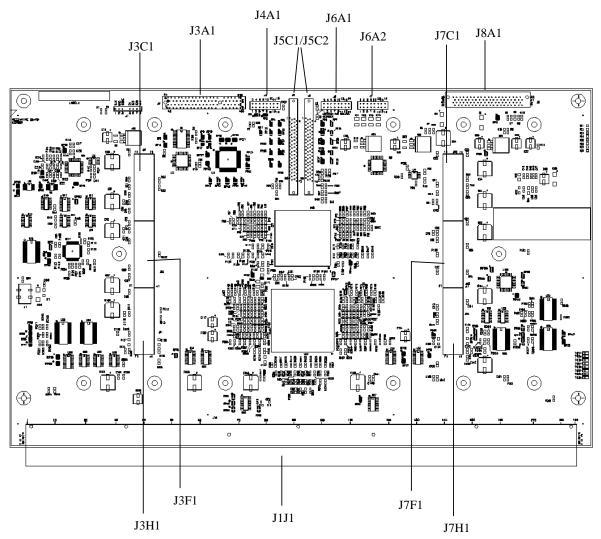
Figure 3-2: Profusion\* Carrier Layout
