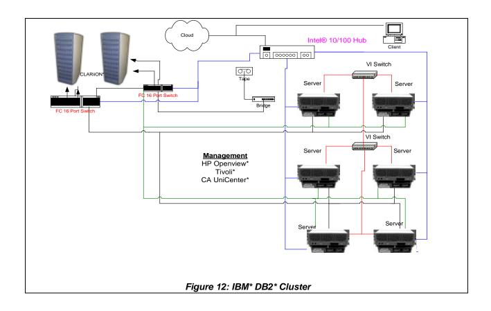
IBM\* DB2\* is a cluster solution where performance is a factor. Six servers with Pentium III Xeon processors power this high performance DB SAN configuration. High Speed Interconnects such as the HAL VI will speed up requested transactions. The FC hubs and switches create the large bandwidths needed to forward the requests made of the server to the storage.
