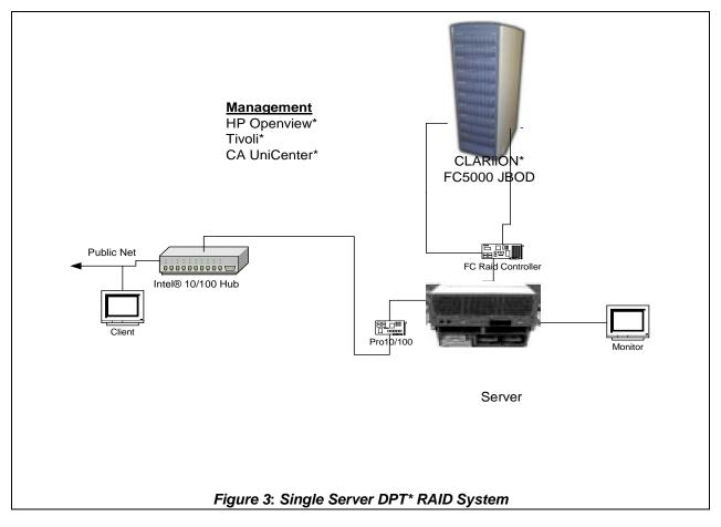
The DPT FC RAID Controller has a Graphical User Interface (GUI) which controls the card. This enables fast setup of RAID configurations and management of the HDD units. The controller is connected to a DAE through both LCCs.
