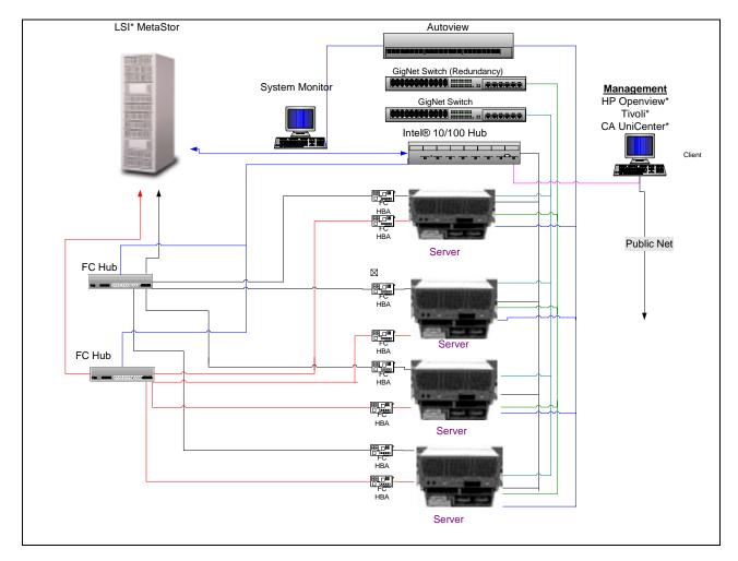
Figure 11: LSI Logic\* MetaStor Oracle\* Parallel Server Cluster
