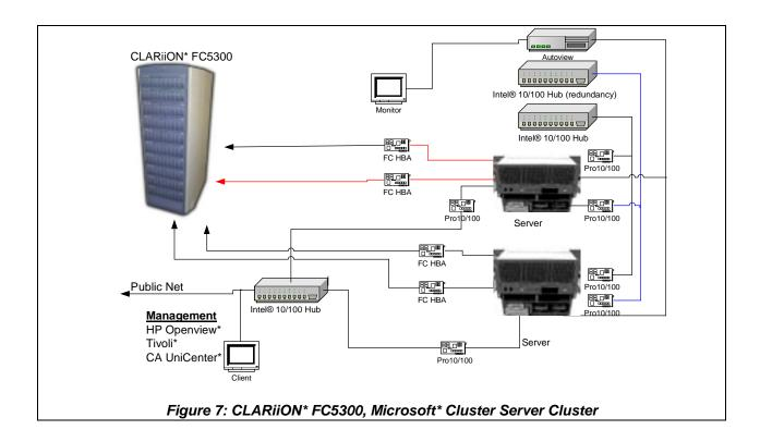
Windows NT 4.0 Enterprise Edition provides all the components needed to run a clustered server solution. In this mode, both servers provide a pool of services and either server can take over the host functions should one server fail to continue reliable operation.
