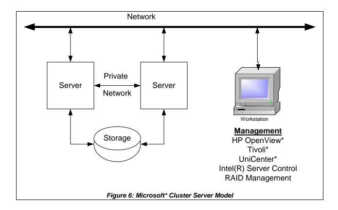
In this model, the private Ethernet network passes "keep alive" information between the two servers. The private network requires two Network Interface Cards (NICs) per server, each NIC is connected to a separate hub. An additional NIC is installed in each system for communication with the public network. A management workstation will manage both servers in the cluster from the public net using HP OpenView, Tivoli, or Unicenter.
