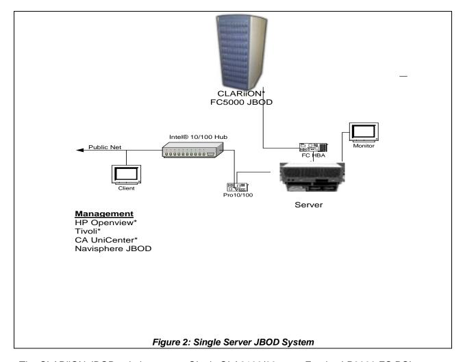
The CLARiiON JBOD solution uses a Qlogic QLA2100/66 or an Emulex LP8000 FC PCI Adapter. The adapter is connected to a CLARiiON Disk Array Enclosure (DAE). The two purposes of the NIC card are to share stored data and provide remote administration by a workstation.
