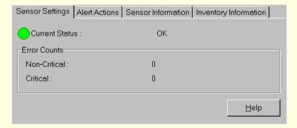
For motherboards that support it, PIC monitors processor failures during runtime and system boot on the managed server. If a supported motherboard includes multiple processors, each processor can be configured and monitored separately through PIC. If a processor failure is detected, the failure is reported as a critical condition in the health branch of the PIC Console software, and the requested event actions are carried out.
