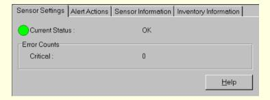
When a chassis door that includes an open/close switch is opened, the vulnerable state is indicated as a critical condition in the health branch of the PIC Console, and the requested event actions are carried out. When all chassis doors that include an open/close switch are closed, PIC indicates the chassis is secure and carries out the requested event actions.
