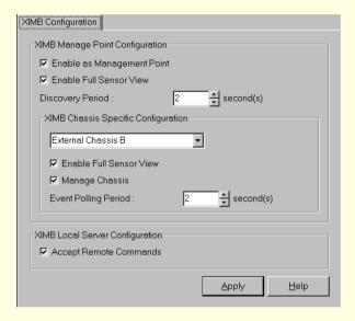
Through the PIC Console, you can switch your view of the primary managed server to one of the ICMB-managed devices and view the available information on that device without losing the connection with the primary server. You can change your view back to the primary server or any other ICMB-managed device at any time. Through the PIC Console, you can configure the ICMB management features of the primary managed server and the remote ICMB-managed devices.
