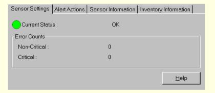
If a power supply reports a predictive failure condition, then PIC reports the status as a non-critical condition in the health branch of the PIC Console software, and the requested event actions are carried out.
