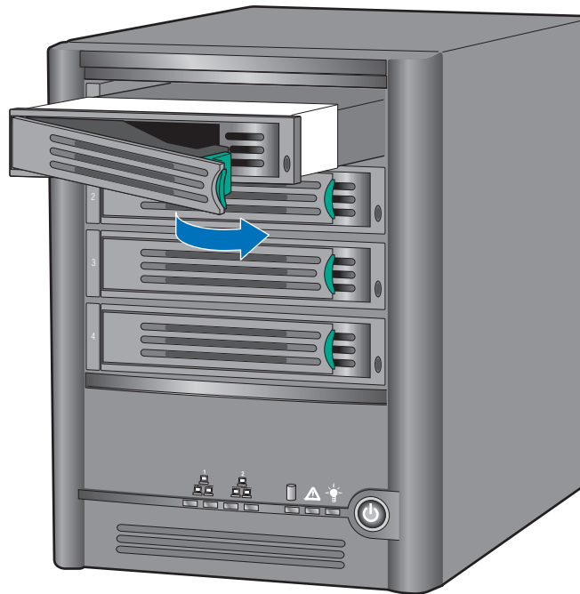
Figure 10. Re-installing Drive Carrier into Storage System
