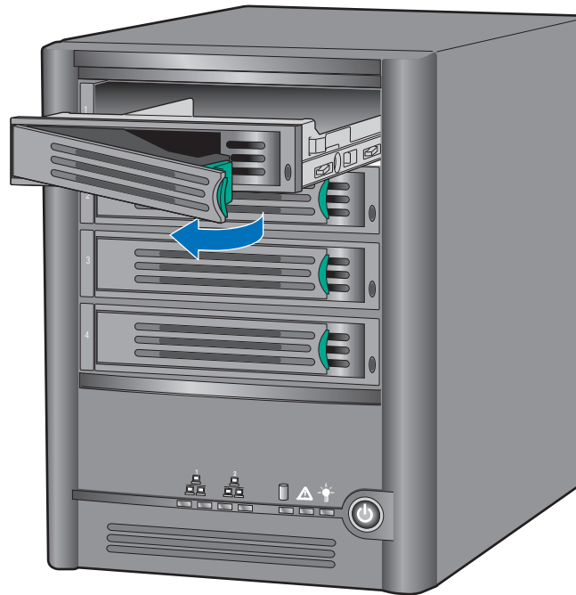
Figure 4. Removing Drive Carrier from Storage System
