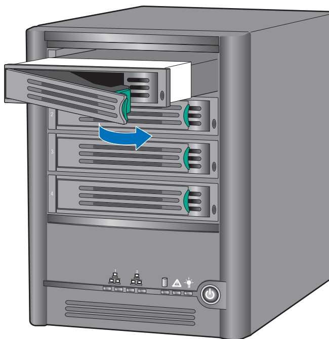
Figure 21. Re-installing Drive Carrier into Storage System
