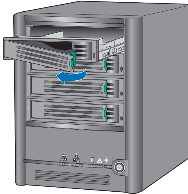
Figure 15. Removing Drive Carrier from Storage System
