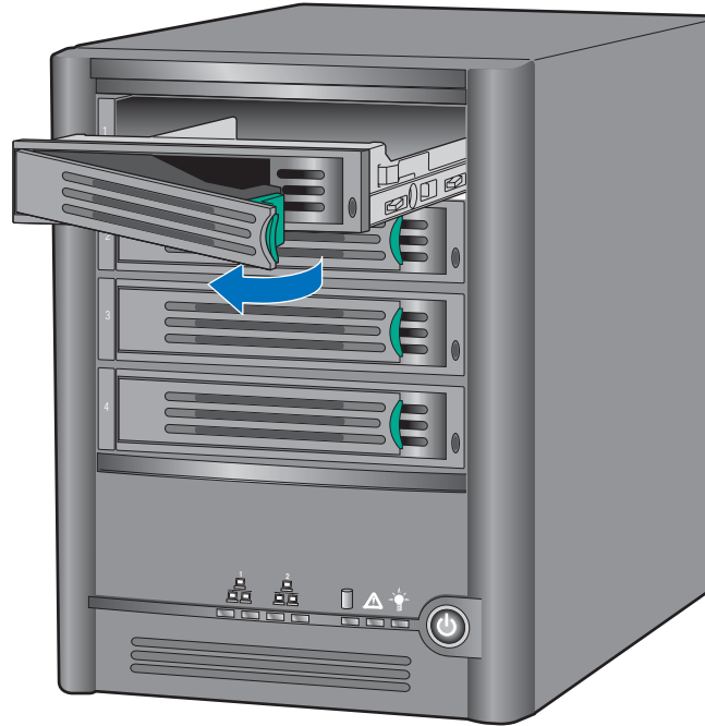
Figure 15. Removing Drive Carrier from Storage System
