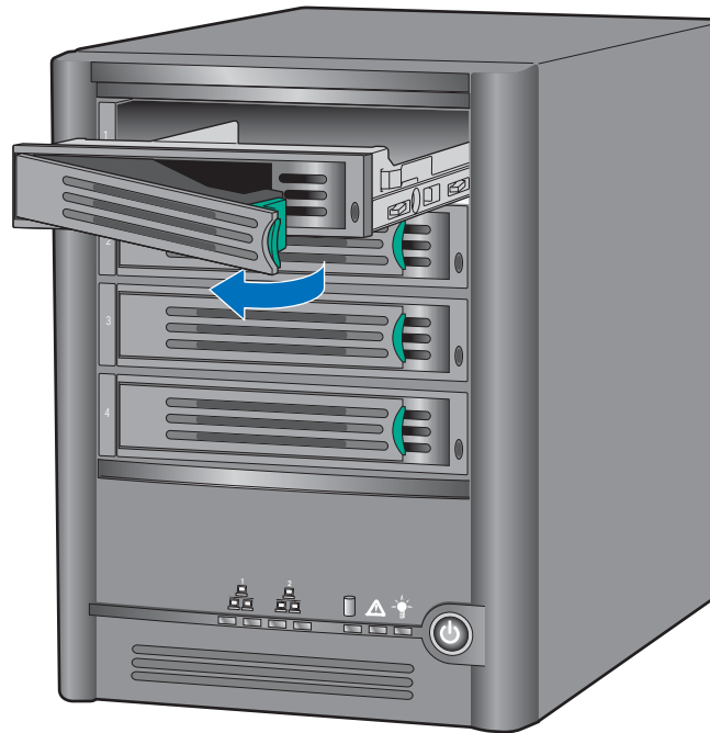
Figure 4. Removing Drive Carrier from Storage System
