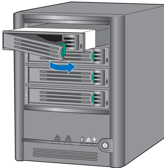
Figure 10. Re-installing the Drive Carrier into Storage System
