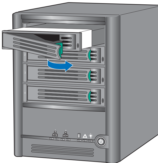
Figure 21. Re-installing Drive Carrier into Storage System
