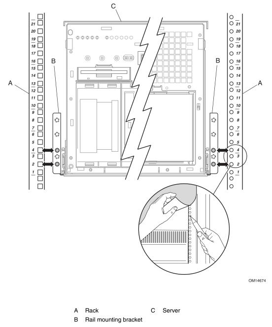
Figure 16. Marking the Mounting Holes for the SPSH4 on the Front of the Rack
