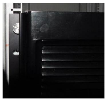
Figure 10. Attaching the Thumbscrews, SRSH4
