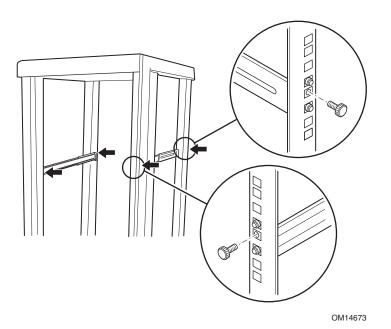
Figure 18. Attaching the Brackets to the Rack
