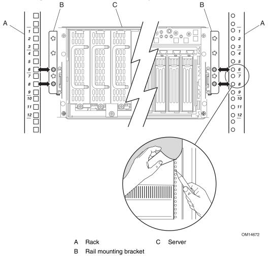
Figure 6. Marking the Mounting Holes for the SRSH4 on the Front of the Rack
