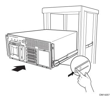
Figure 19. Installing the SPSH4 Server into the Rack
