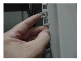
Figure 17. Attaching Clipnuts to the Rack
