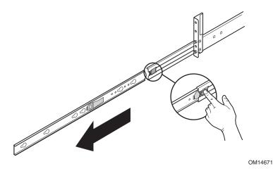
Figure 13. Removing the Inner Rails
