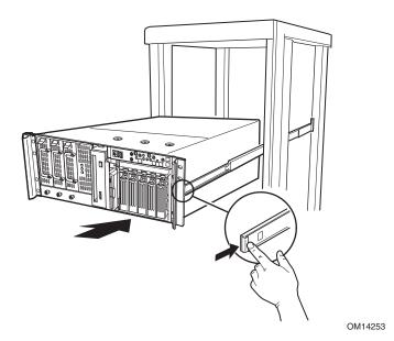
Figure 9. Installing the SRSH4 Server into the Rack
