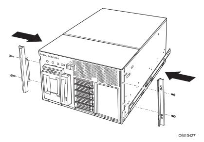
Figure 15. Installing the SPSH4 Rack Pull Handles
