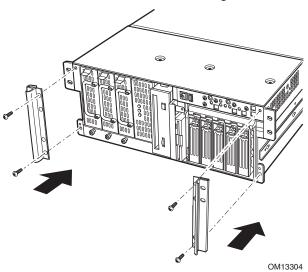
Figure 5. Installing the SRSH4 Rack Pull Handles
