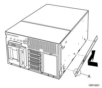
Figure 14. Attaching the Inner Rails to the SPSH4 Chassis
