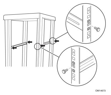
Figure 8. Attaching the Brackets to the Rack
