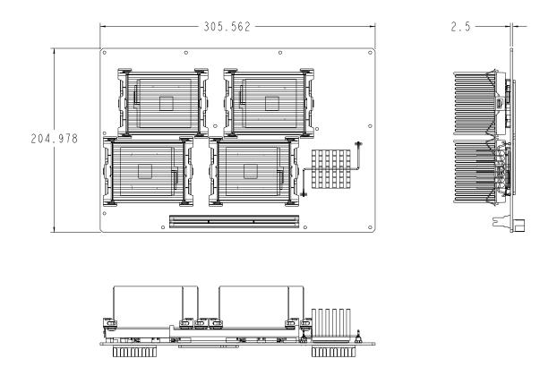
Figure 25. Processor Board Mechanical Diagram
