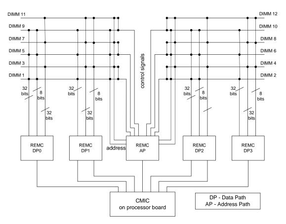
Figure 6. Memory Block Diagram
