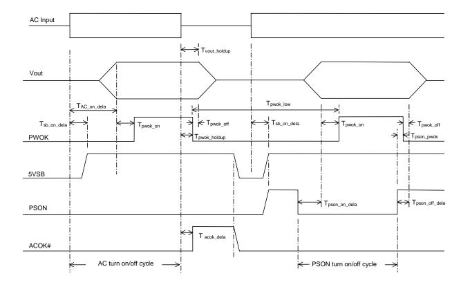
Figure 22 Turn On Turn Off Timing
