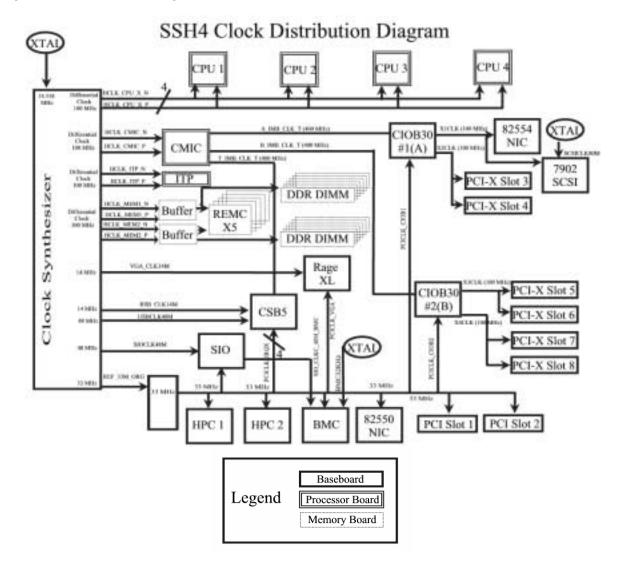
Figure 14 illustrates clock generation and distribution on the baseboard.
