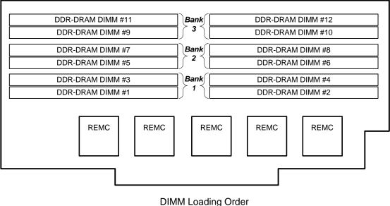
Bank 1: DIMMs 1, 2, 3, and 4 Bank 2: DIMMs 5, 6, 7, and 8 Bank 3: DIMMs 9, 10, 11, and 12
