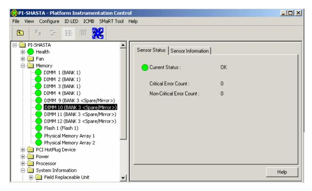
Figure 8 Advanced Mirror Memory Configuration status Tab (Normal
