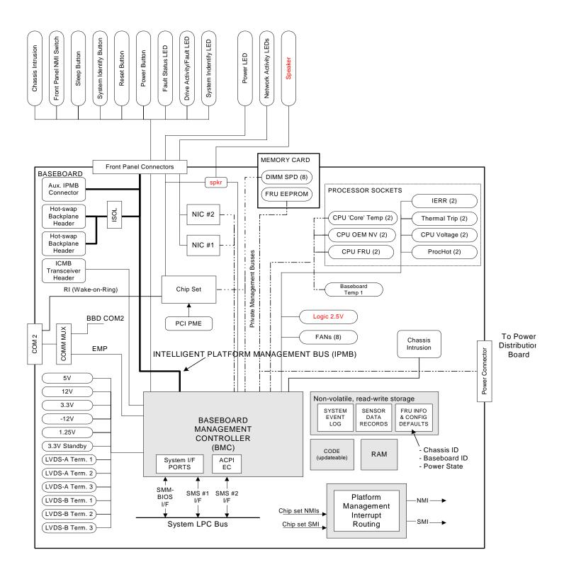
Figure 13. SSH4 Sahalee BMC Block Diagram
