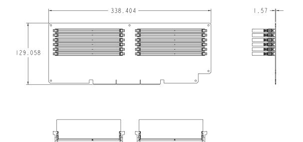
Figure 24. Memory Board Mechanical Diagram
