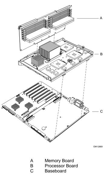
Figure 1. Baseboard, Processor Board, and Memory Board
