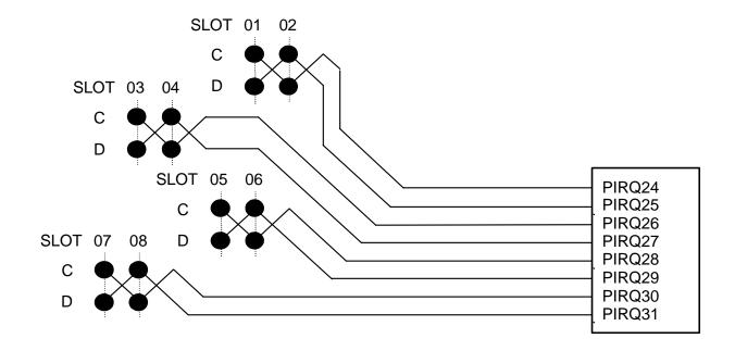
Figure 4. Interrupt Routing (Symmetric Mode)
