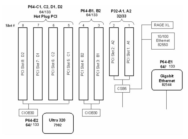
Figure 2. PCI Bus Layout
