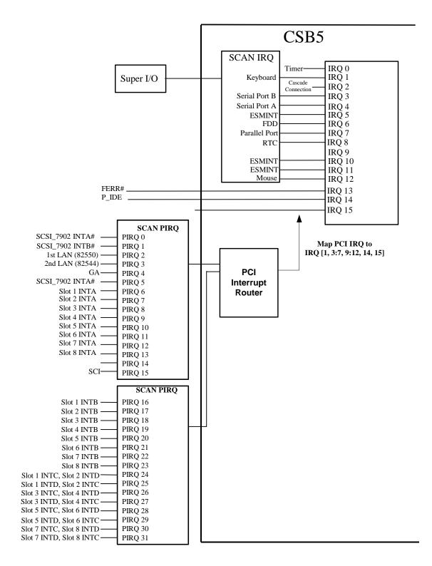
Figure 3. Interrupt Routing (PIC Mode)
