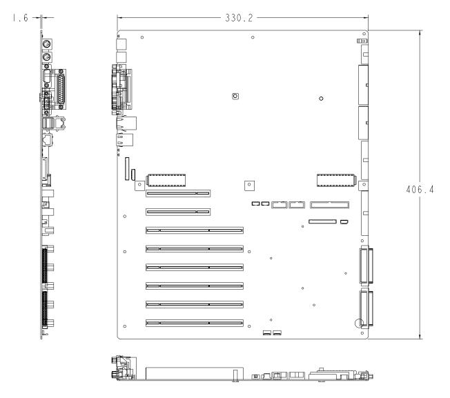
Figure 23. Baseboard Mechanical Diagram
