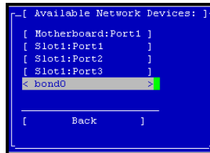
Figure 207. Selecting a Bonded Interface in the Available Network Devices Window
