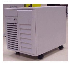
Figure 2-1 Chenbro A9891-207 ATX Net Server Chassis
