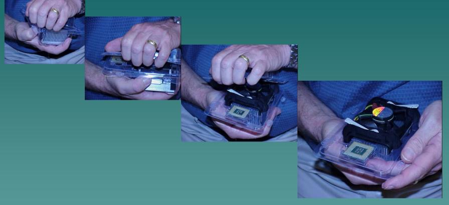
Maintain grip on FHS from underneath in one hand & palm top of FHS with other hand and work both lift points first by prying with fingers at each corner until clamshell pressure is released. You may have to apply same method to opposite two corners in order to ensure complete release. You may hear a slight pop or feel a slight pop; this is normal and signifies that the pressure has been released.
