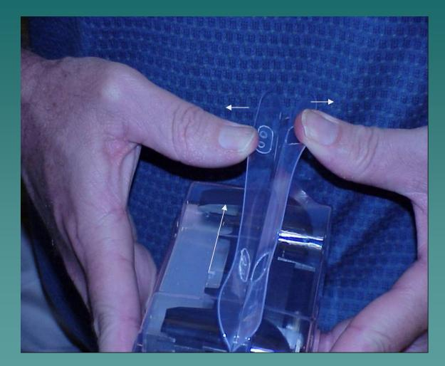
Once Weld #1 & #3 are broken, reorient clamshell so that the FHS is between both hands on lap with CPU towards stomach and weld # 2 and # 4 are up. Repeat steps to break welds 2 & 4 by prying lid and tray flanges away from each other with thumbs while holding clamshell between both hands by the FHS. See Diagram #1 and Diagram #2 at the end of this document.
