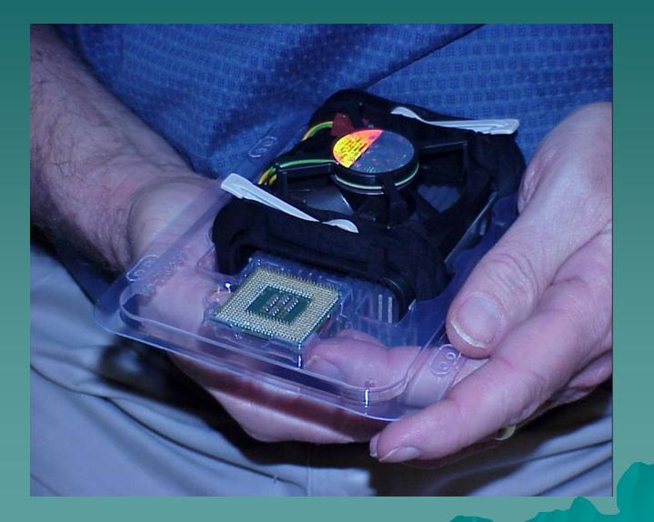
Carefully, lift the lid off the container while maintaining grip from underside (tray side) of the FHS. Optional to set clam shell onto tabletop with hologram facing up and lift lid. The processor should be carefully lifted from the tray using the semi-circle indents to grab the green edges of the substrate of the processor.
