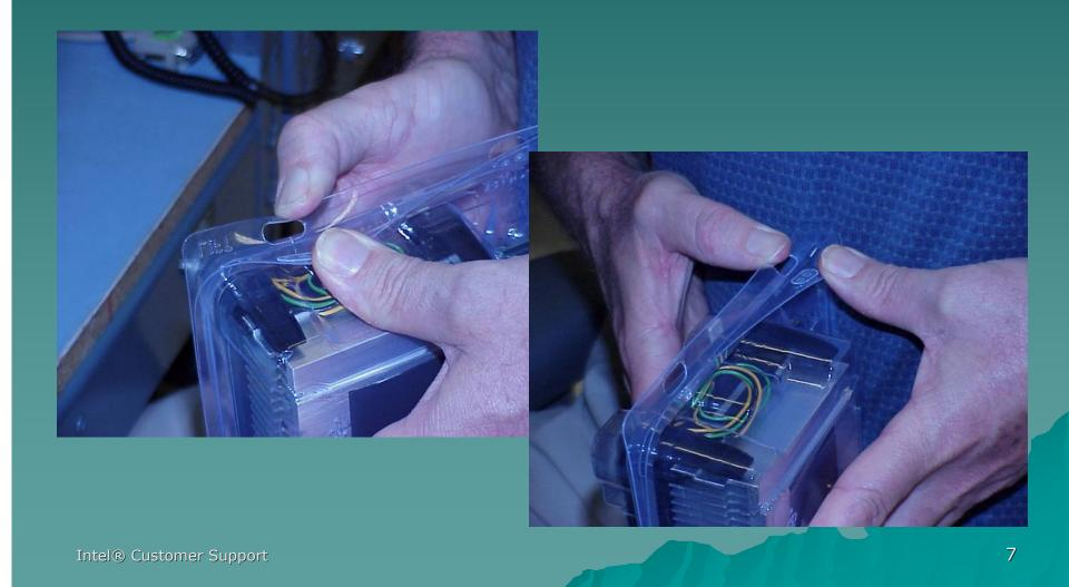
Once all four welds are broken, hold clamshell in either hand from underside of FHS so that the Intel® hologram is facing up and the container will have the embossed "Intel" showing. (Lid up) See Diagram #2 at the end of this document.
