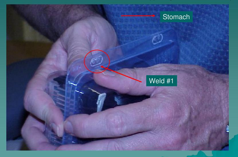
Locate the two corners of the plastic container marked "LIFT" on weld #1. These are found on the two corners closest to the FHS.
