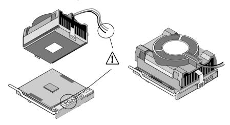
It is important that the Intel<sup>®</sup> Pentium<sup>®</sup> III processor fan heatsink aligns properly with the 370-pin socket. Make sure to align the processor fan heatsink with the socket base as shown above. This will align the fan cable with the PGA370 mark on the 370-pin socket. Proper alignment will ensure correct processor operation.
