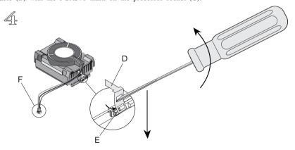
Attach the fan heatsink clip (D) to the processor socket (E). Connect the processor fan cable header (F) to the motherboard connector.
