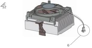
Snap the fan on the heatsink. Fan orientation is not important. Connect the processor fan cable header (G) to the motherboard connector.
