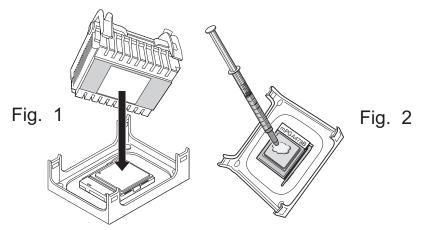
The heatsink may have thermal interface material attached to the bottom as shown in Fig. 1. (Be careful not to damage the thermal interface material.) If not, use the enclosed syringe and apply all of the thermal interface material to the top of the processor as shown in Fig. 2.
