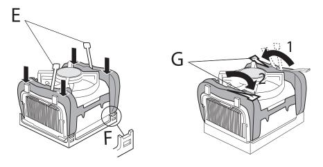
Align the heatsink and clip assembly with the retention mechanism and place it on the processor. The heatsink is symmetrical. With the clip levers in the up position (E), push down on all four clip frame corners to secure to the retention mechanism hooks (F). Close the clip levers (G) (levers require force to be completely closed).
