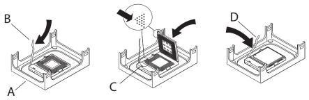
Install the processor retention mechanism (A) following the motherboard manufacturer's installation instructions. Open the socket handle (B). Install the processor by carefully aligning the pins to the socket (C). Close the socket handle (D).
