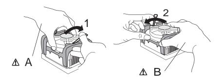
When installing the fan heatsink and clip assembly, it is important to not allow the heatsink to rotate or twist on the processor. Securing the fan heatsink while closing the clip levers will ensure the thermal interface material is not damaged and the processor will operate correctly (the thermal interface material, between the processor and heatsink, is attached to the heatsink).
