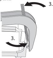
3. Push down on the clip hook and simultaneously rotate the screwdriver towards the fan heatsink to free the clip hook from the retention mechanism (RM). Repeat this process for the remaining clip hooks. Then, remove the fan heatsink.
