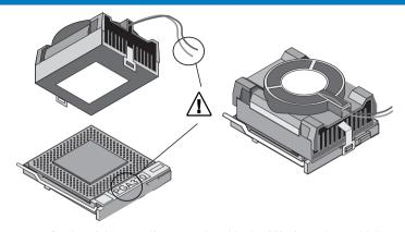
The processor fan heatsink must align properly with the 370-pin socket. Make sure to align the fan heatsink with the socket base as shown above. This will align the fan cable with the PGA370 mark on the socket.
