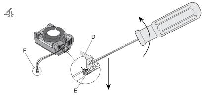
Attach the fan heatsink clip (D) to the processor socket (E). Connect the processor fan cable header (F) to the motherboard connector.
