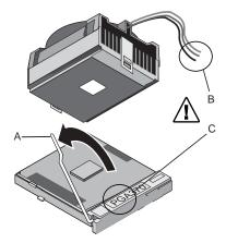
With the processor in the socket, close the handle (A). Place the fan heatsink on top of the processor. Be careful not to damage the thermal interface material. Align the fan cable (B) with the PGA370 mark on the processor socket (C).
