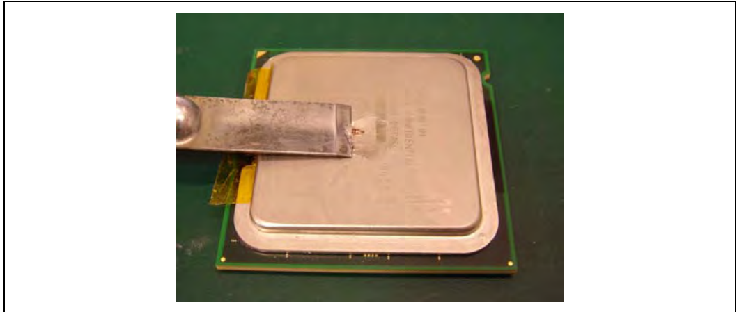
Figure 7-35. Removing Excess Adhesive from IHS
