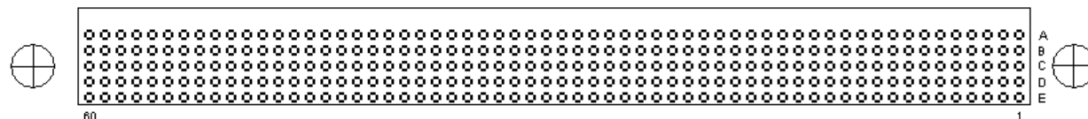
Figure 5-17. CPU Baseboard Memory Connector Pin Diagram
