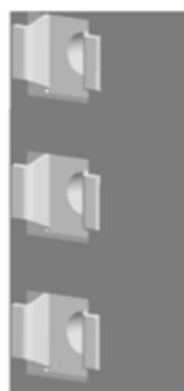
Figure 1-10. Clip Nut Orientation
