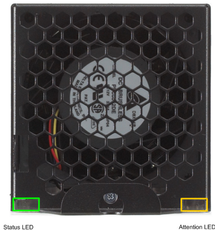
Figure 1-61. 12800 Fan LEDs
