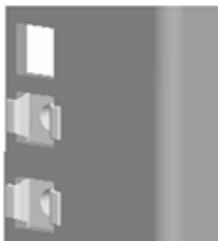
Figure 1-14. Clip Nut Orientation
