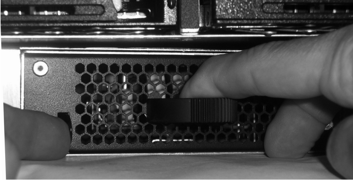
Figure E-5 12300 Fan/Power Module Removal
