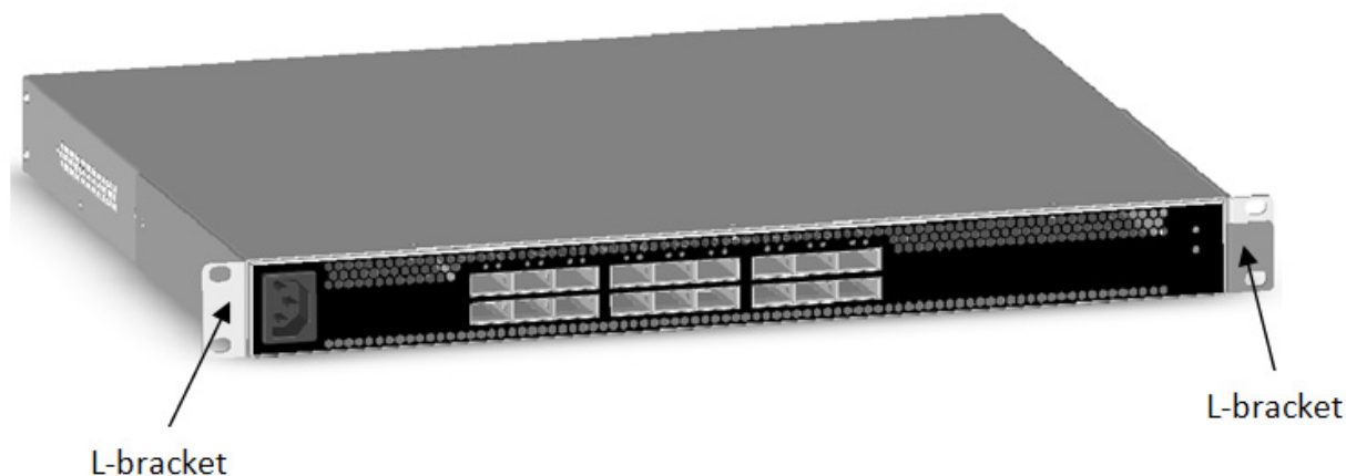
Figure 1-8. 12200 Two Post Installation
