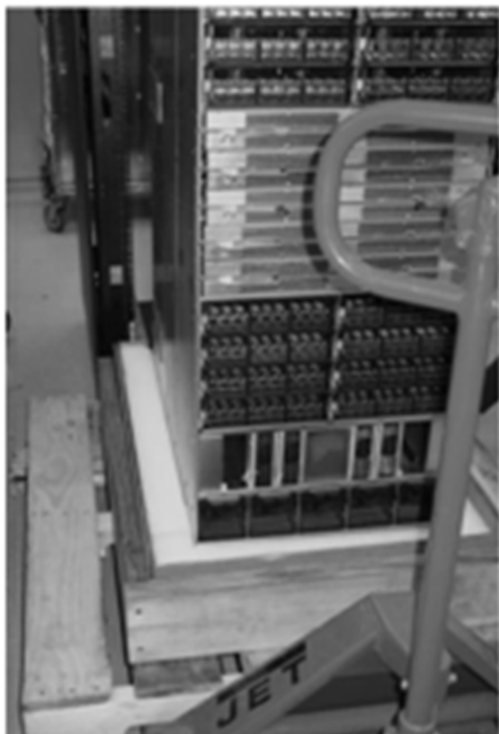
Figure 1-36. Sliding the Switch off the Pallet
